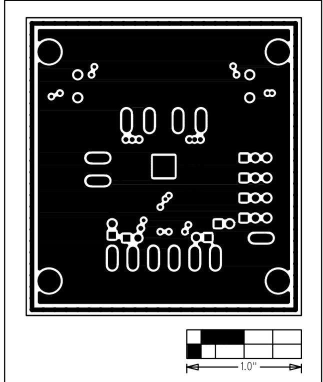
Figure 5. MAX9714 EV Kit PC Board Layout—Layer 3 (VDD)
