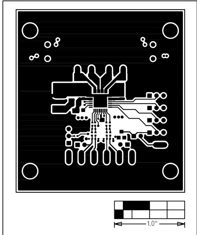
Figure 3. MAX9714 EV Kit PC Board Layout—Component Side
