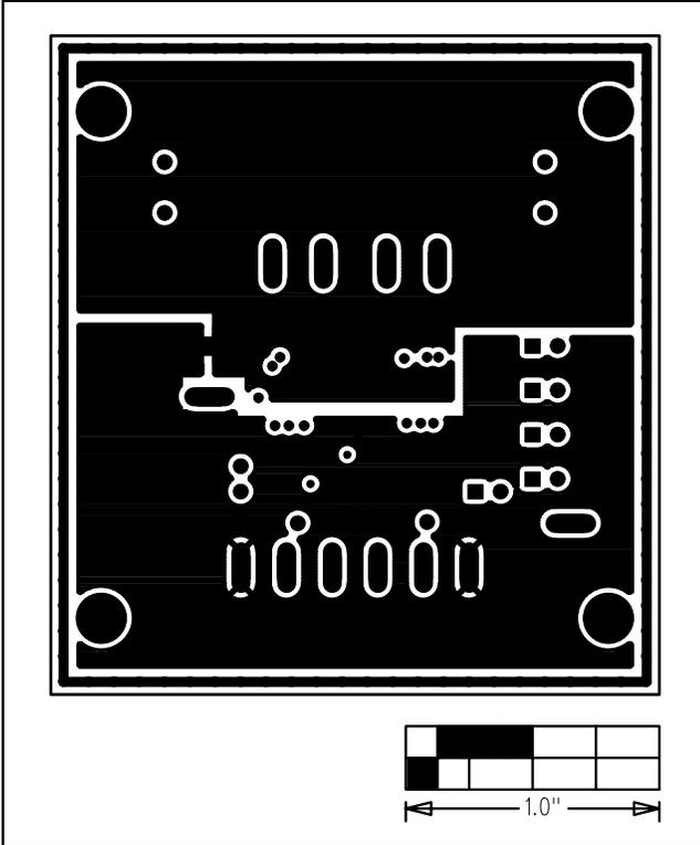
Figure 4. MAX9714 EV Kit PC Board Layout—Layer 2 (GND)
