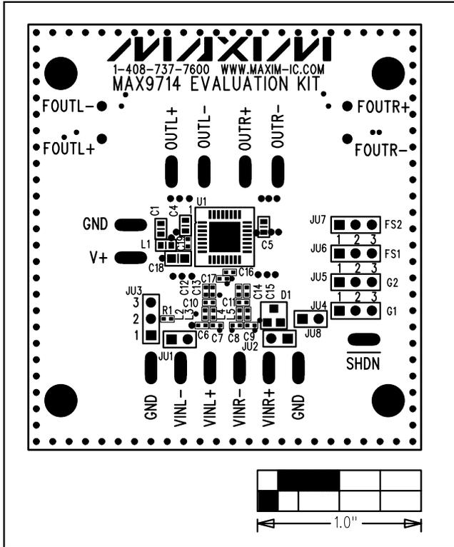
Figure 2. MAX9714 EV Kit Component Placement Guide—Component Side
