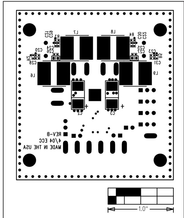
Figure 7. MAX9714 EV Kit Component Placement Guide—Solder Side
