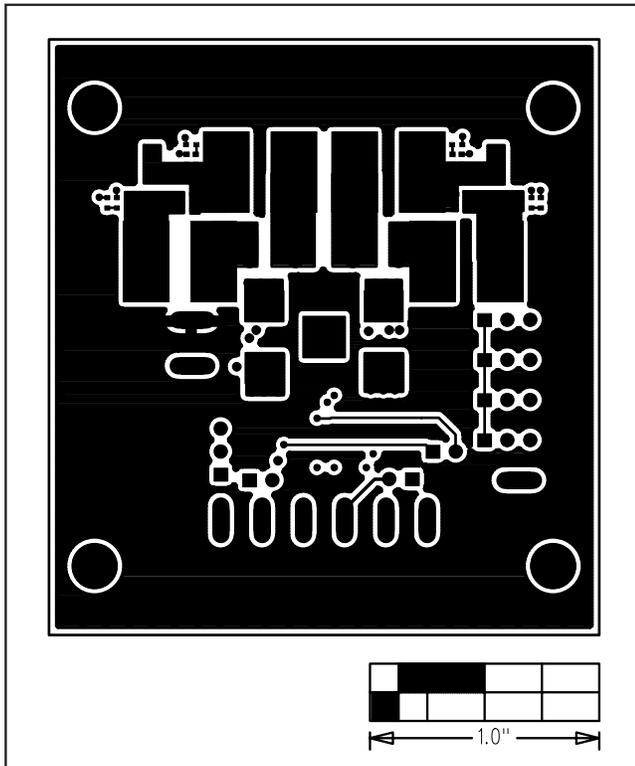
Figure 6. MAX9714 EV Kit PC Board Layout—Solder Side
