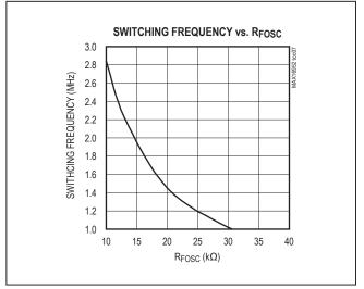
Figure 3. Switching Frequency vs. R<sub>FOSC</sub>
