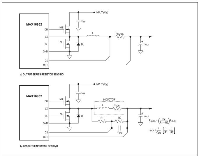
Figure 4. Current-Sense Configurations
