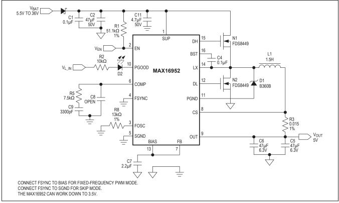
Figure 6. Typical Operating Circuit for  $V_{OUT} = 5V$
