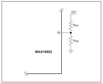
Figure 2. Adjustable Output Voltage
