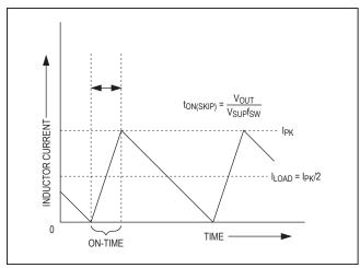
Figure 1. Pulse-Skipping/Discontinuous Crossover Point
