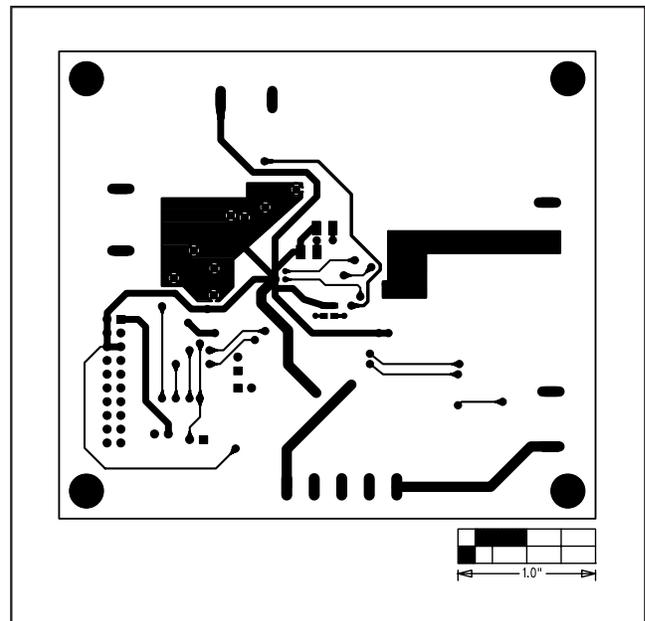
Figure 9. MAX1645B EV Kit PC Board Layout—Solder Side
