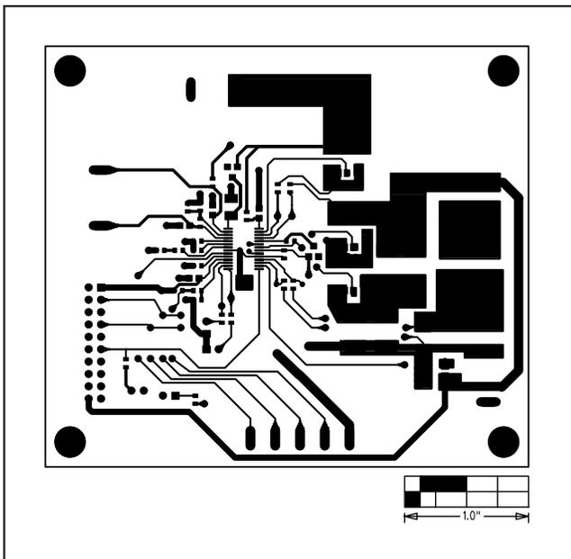
Figure 8. MAX1645B EV Kit PC Board Layout—Component Side
