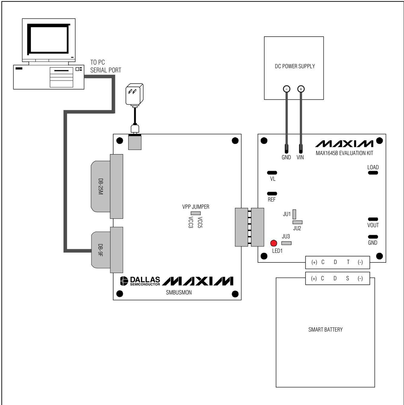
Figure 1. Block Diagram of MAX1645B EV System
