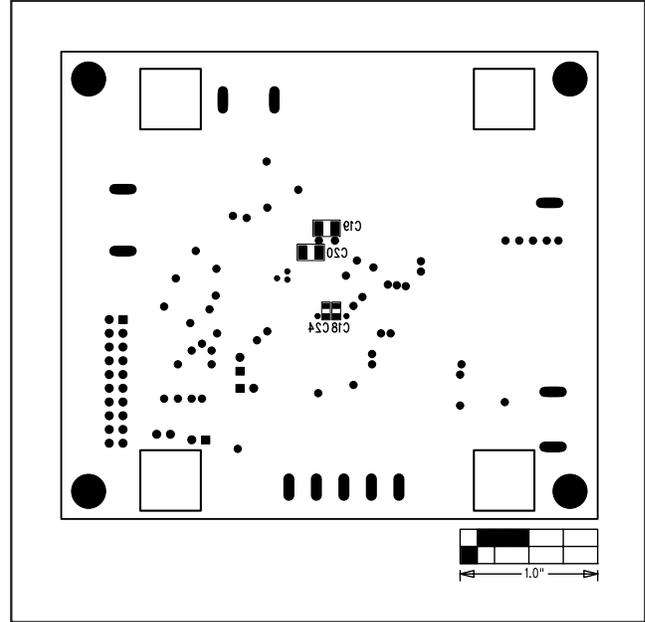
Figure 7. MAX1645B EV Kit Component Placement Guide—Solder Side
