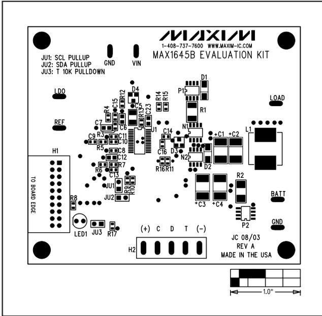
Figure 6. MAX1645B EV Kit Component Placement Guide—Component Side
