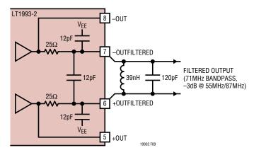
Figure 9. LT1993-2 Output Filter Topology Modified for Bandpass Filtering (1 External Inductor, 1 External Capacitor)
