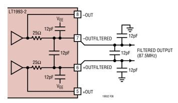
Figure 8. LT1993-2 Internal Filter Topology Modified for 1/2x Filter Bandwidth (3 External Capacitors)
