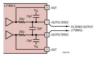
Figure 6. LT1993-2 Internal Filter Topology -3dB BW ≈175MHz
