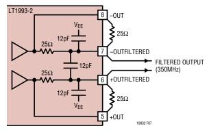
Figure 7. LT1993-2 Internal Filter Topology Modified for 2x Filter Bandwidth (2 External Resistors)
