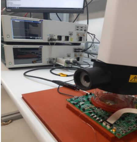
Figure 6. DDR3L Compliance Testing Setup
