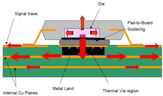
Fig. 1 Cross-section of exposed pad pkg with heat transfer
