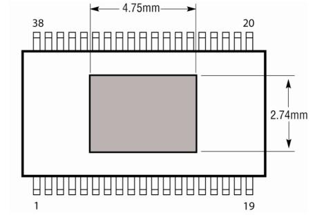
Fig 2. Example: 38L TSSOP exposed pad pkg bottom view
