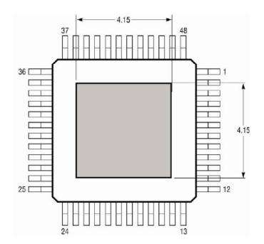
Fig 3. Example: 48L LQFP exposed pad package bottom view
