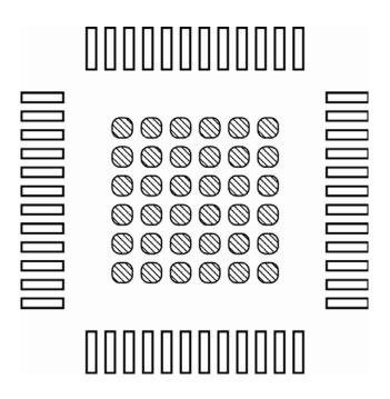
Fig 6. Recommended stencil design for LQFP
