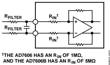
Figure 1. Analog Input Circuitry
