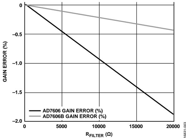
Figure 2. Gain Error Introduced by the Input Series Resistor ( $R_{FILTER}$ )
