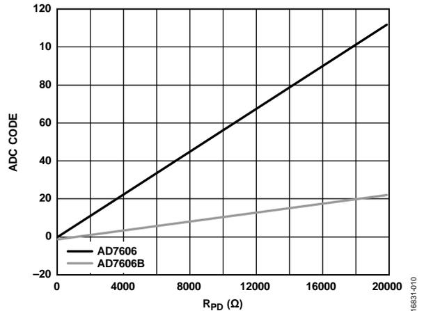
Figure 4. ADC Output Code When the Sensor Disconnects vs. the  $R_{PD}$  Value
