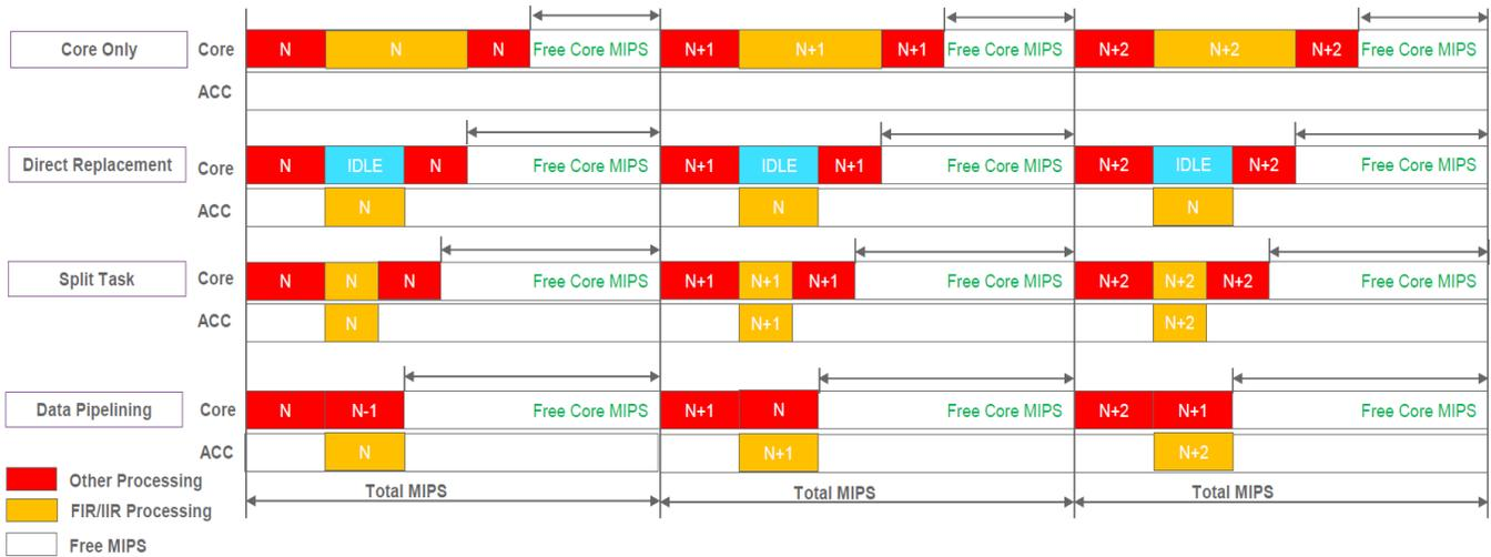
Figure 13: Accelerator Usage Models
