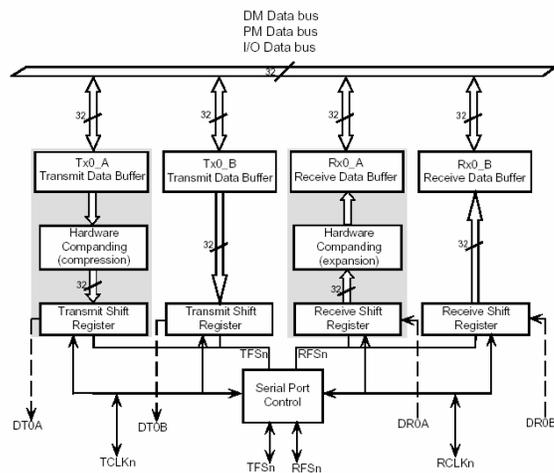
Figure 1. Serial Port Block Diagram
