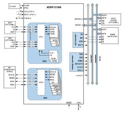
Figure 3. ADSP-21368 system sample configuration
