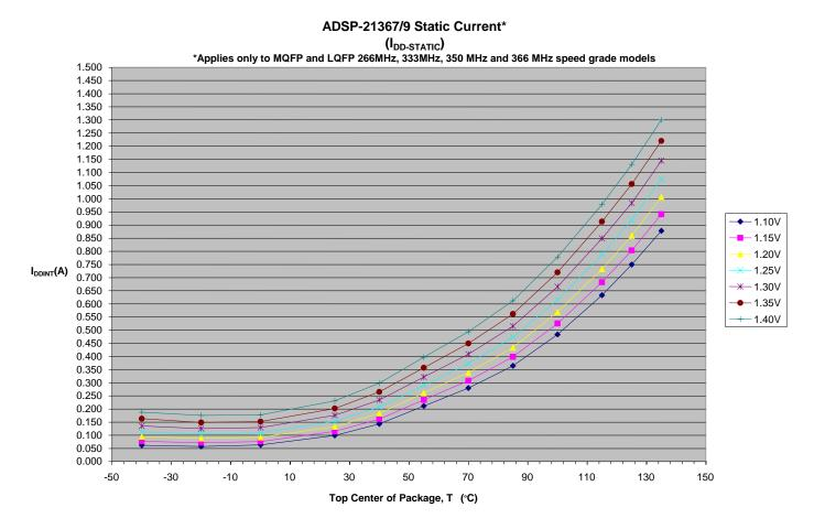
Figure 5. I<sub>DD-STATIC</sub> graph
