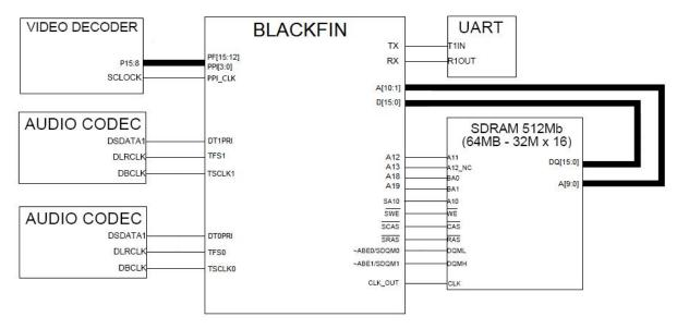
Figure 6. Blackfin System Sample Configuration
