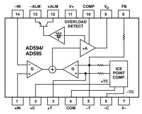
Figure 2. AD594/AD595 Functional Block Diagram
