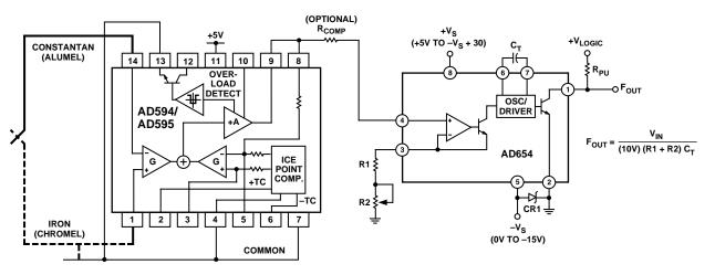
Figure 8. Temperature-to-Frequency Conversion
