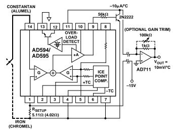
Figure 7. Current-Mode Transmission
