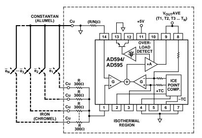
Figure 10. Measuring Average Temperature
