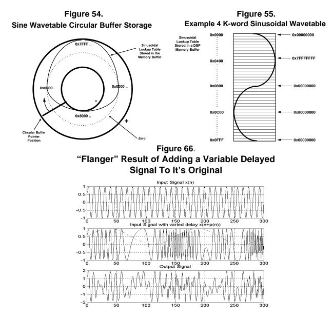
This sinusoidal LFO's frequency is usually controlled by the '*sweep rate*' parameter. The LFO can easily be implemented on the DSP by creating a sine wavetable lookup that determines the variation of the delay time. The determination of the delay time can be updated periodically using the on chip programmable timer.
