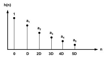
The difference equation is a simple modification of the single delay case. To 5 delays of the input (see Figure 43), the DSP processing algorithm would perform the following difference equation operation:
