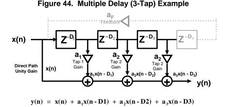
The above structure uses 3 delay-line tap points for fetching samples. In addition, feedback can be used to take the output of the system delay and feed it back to the input.
