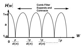
The Frequency Response of the Flanger results in a Comb Filter. As the Delay Increase, the number of peaks increases. Changing the Delay modifies the comb filter, which in turn affects the frequencies that are enhanced or cancelled.
