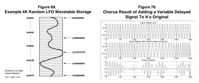
A result of an increasing slope in the LFO will cause the pitch to be lower. A negative slop will result in a pitch increase. The LFO value in the table can be updated on a sample basis via the chorus processing routine, or the wavetable look-up can be modified using the DSP's on-chip programmable timer. The varying delay d(n) will be updated using the following equation:
