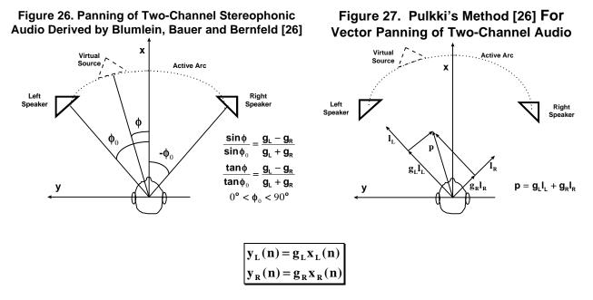
To create a panning effect of an audio channel to a particular position in the stereo output field, the programmer can use the Stereophonic Law of Sines, or the Tangent Law equation (Pulkki, Blumlein and Bauer[22].. see Figure 26) where  $g_L$  and  $g_R$  are the respective gains of the left and right channels.
