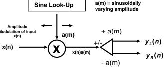
For Stereo Tremolo: when a(m) > 0 x(n)a(m) panned to left channel right channel is zero when a(m) < 0 x(n)a(m) panned to right channel left channel is zero Example Stereo Tremolo Implementation on the ADSP-21065L
