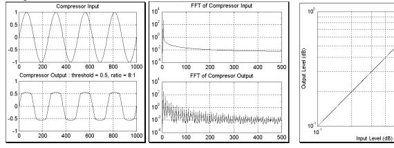
**Compressor Characteristics : threshold = 0.5, ratio = 20:1**
