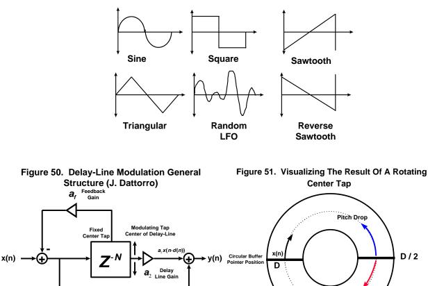
Figure 49. Common Methods of Modulation
