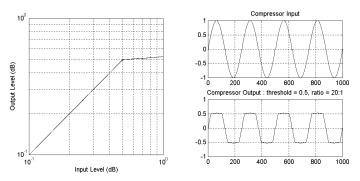
The following code example is a stereo limiter with a ratio of  $1:\infty$  - in other words, it clips the signal at a certain threshold. As seen below, this is extremely simple to do using the **clip** function.
