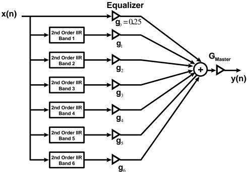
Figure 33. DSP Implementation of a 6-Band Digital Graphic
