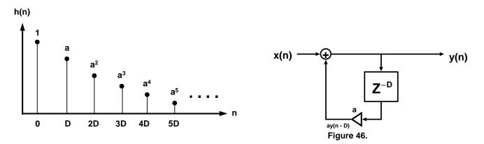
Adding an infinite # of delays will create a rudimentary reverb effect by simulating reflections in a room (Figure 46). The difference equation then becomes and IIR comb filter (Figure 46):
