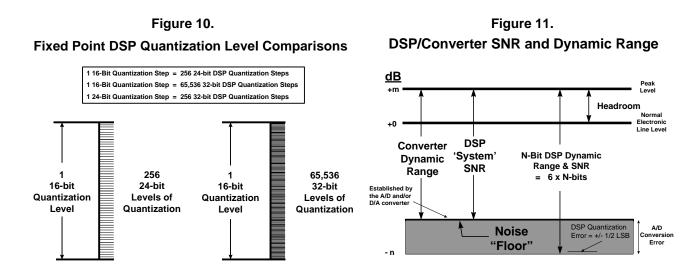
The maximum representable signal amplitude to the maximum quantization error for of an ideal A/D converter or DSP-based digital system is calculated as:
