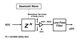
Figure 74. Implementation of a Generic Pitch Shifter
