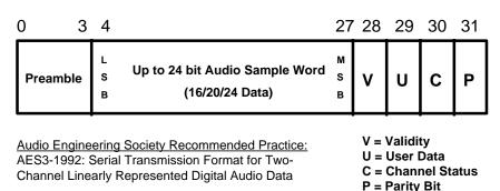
*SPD/IF* (*Sony/Philips Digital Interface Format*) is based on the AES/EBU standard in operating in 'consumer' mode. The physical medium is an unbalanced RCA cable. The consumer mode carry less control/status information. Typical applications where this interface can be found is in home theater equipment and CD players.
