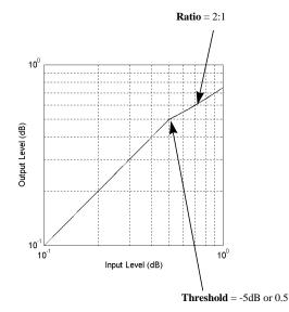
There are two primary parameters for a compressor : threshold and ratio. The threshold is the signal level at which the gain reduction begins and the ratio is the amount of gain reduction that takes place past the threshold. A ratio of 2:1, for example, would reduce the signal by a factor of two when it passed the threshold level as seen in the first compressor example below.
