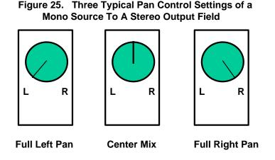
Many 4/8/12 track analog and digital studios contain a knob to pan an input source entirely to the left or right channel, or played back through both channels at an equal mix (with the pan control centered in the middle). To give the listener a sense of location within the output stereo filed, the DSP can simply perform a multiplication of the algorithmic result on both the left and right channel so that it is perceived from coming from a phantom source.
