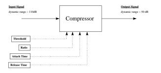
Compressors are used to 'compress' the dynamic range of a signal
