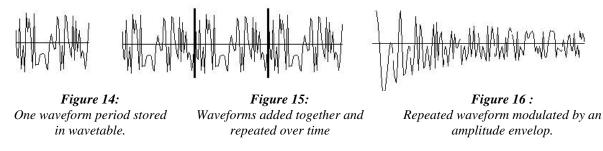
This method of synthesis is simple to implement and is computationally efficient. In a DSP, the desired waveforms can be loaded into a circular buffers to allow for zero-overhead looping. The only real computational operations will be adding multiple waveforms, calculating the amplitude envelope and modulating the looping sample with it. The downside of wavetable synthesis is that it is difficult to approximate rapidly changing spectra.[1]
