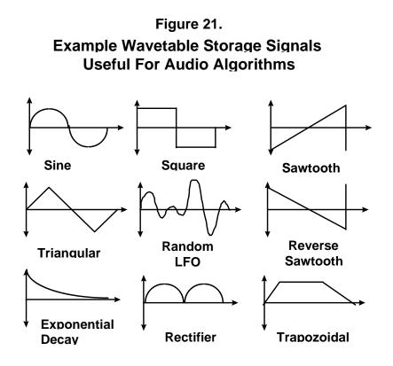
Most high level languages such a C/C++ have build in support to generate trigonometric functions. Real-time Embedded System Software Engineers who program DSP algorithms mostly in assembly do not have the flexibility of a high level language when generating signals. Various methods proposed by Crenshaw [8], Orfanidis [2] and Chrysafis [39] can be used for generating sinusoidal/random signals in a DSP. Signal generation can be achieved by:
