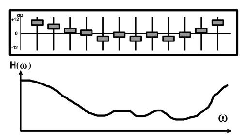
Analog equalizers typically uses passive and active components. Increasing the number of bands results in a large board design. When implementing the same system in a DSP, however, the number of bands is only limited by the speed of the DSP (MIPs) while board space remains the same. Resisters and capacitors are replaced by discrete-time filter coefficients, which are stored in a memory and can be easily modified.
