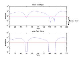
The following code example is a stereo noise gate. This algorithm turns off the signal if its amplitude is below a certain level using RMS level detection of a signal to determine if the signal itself should be turned on or not.
