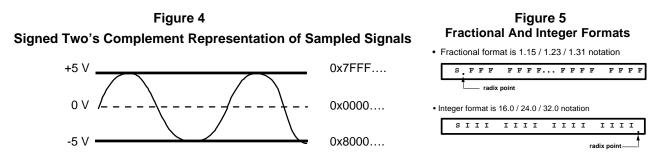
In the fractional format, the binary point is assumed to be to the to the left of the LSB (sign bit). In the integer format, the binary point is to the right of the LSB (figure 5).
