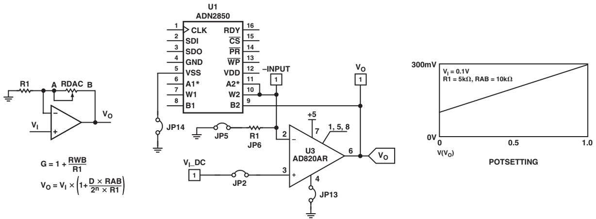
Figure 6. Noninverting Linear Gain
