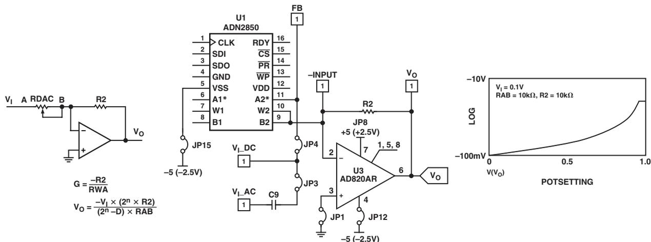
Figure 5. Inverting Exponential Gain and Attenuator
