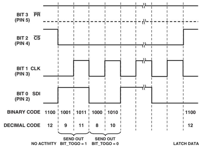
Figure 12. Timing Definition (For VB Program Developers Only)
