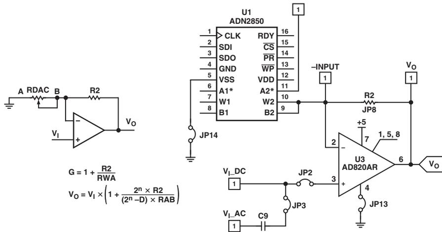
Figure 7. Noninverting Exponential Gain
