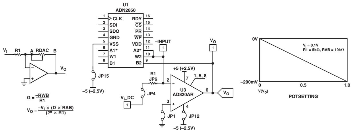
Figure 4. Inverting Linear Gain and Attenuator
