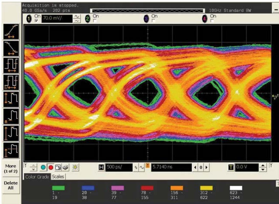
Figure 5. PRBS mode—eye diagram (15m cable with 1.1dB preemphasis setting).
