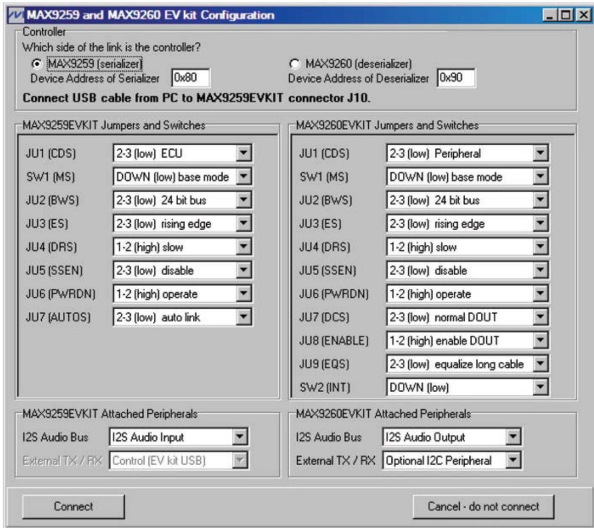
Figure 2. MAX9259/60 EV kits software configuration window.
