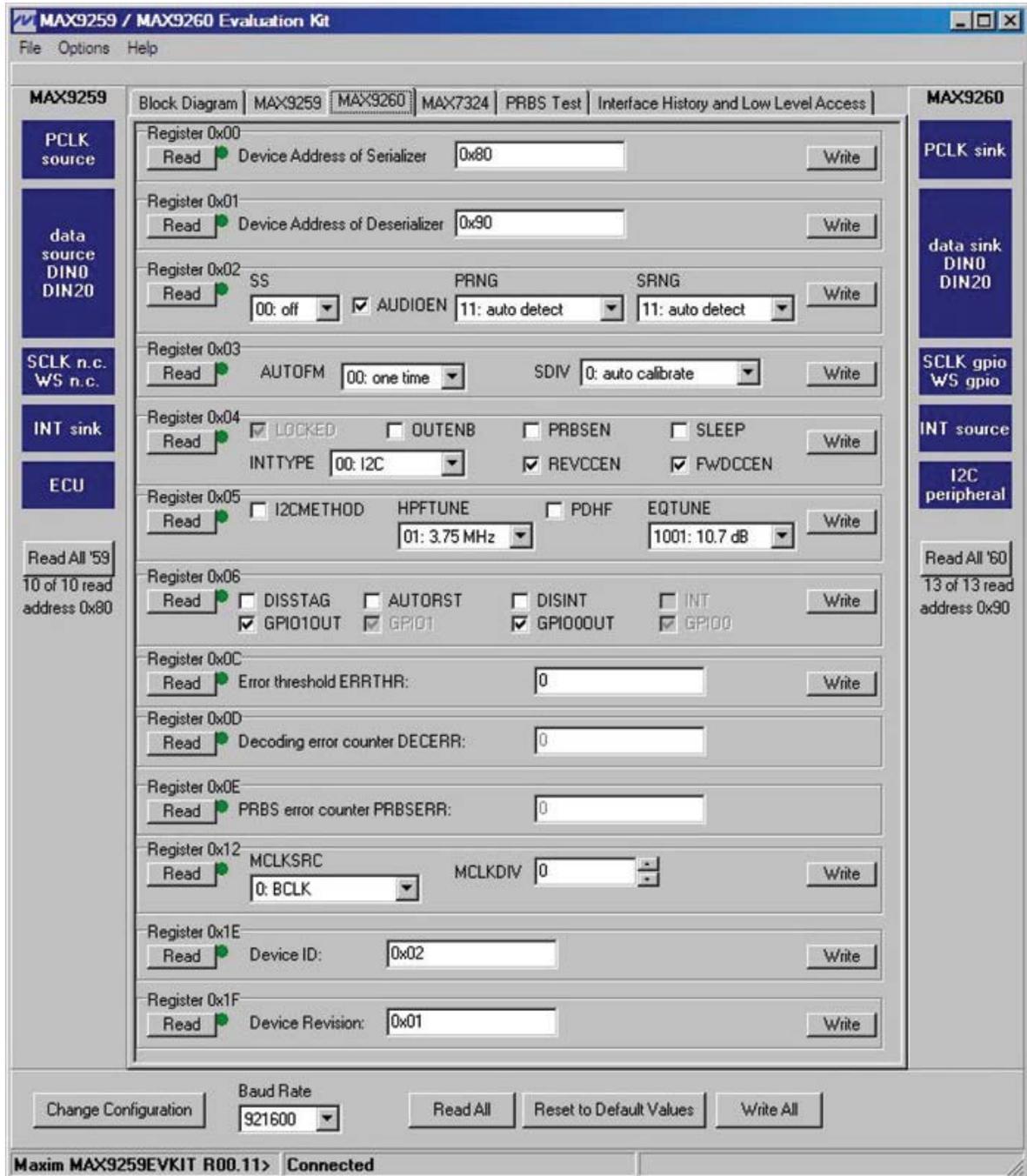
Figure 4. MAX9259/MAX9260 EV kits software main window (MAX9260 tab).
