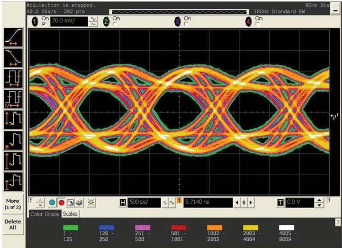
Figure 6. PRBS mode—eye diagram (15m cable with 10.5dB preemphasis setting).
