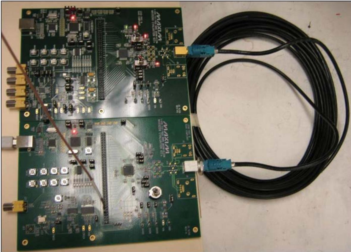
Figure 1. MAX9259/MAX9260 EV kits with 15m STP cable bench setup.
