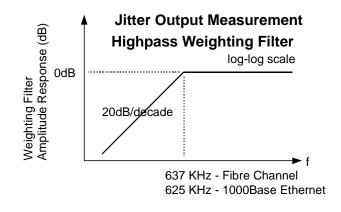
Figure 4. Jitter output measurement using a highpass weighting filter
