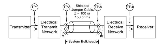
Figure 6. Serial link using shielded jumper cable
