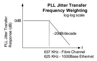
Figure 9. PLL jitter transfer using lowpass frequency weighting
