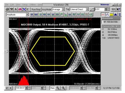
Figure 7. Eye-diagram display
