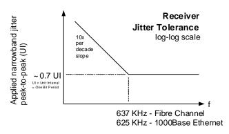
Figure 3. Characteristic receiver jitter tolerance
