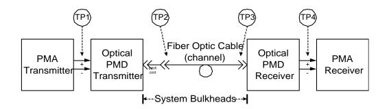
Figure 5. Serial link using fiber optic cabling
