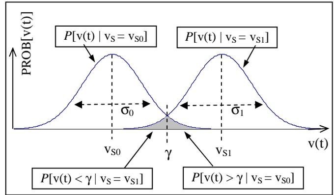
Figure 2. Probability of error for binary signaling
