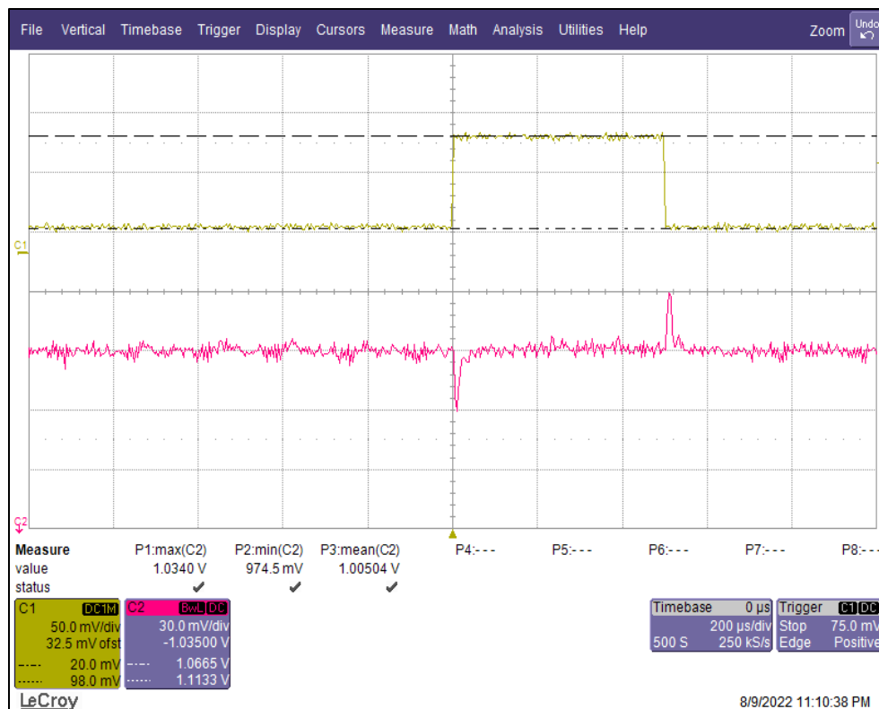
Figure 9a. Shows uncompensated s/m with C_{out}=1600\mu F .
