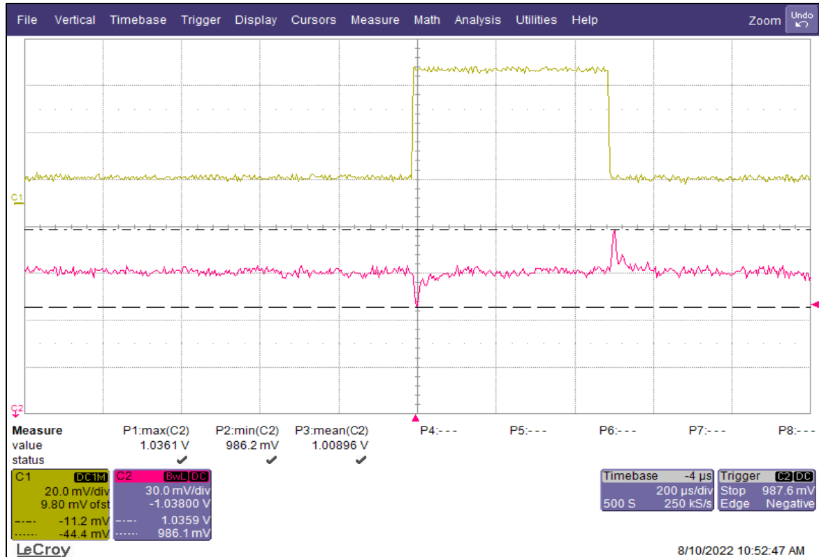
Figure 11b. Shows Lead compensated s/m with C_{out}=870\mu F .
