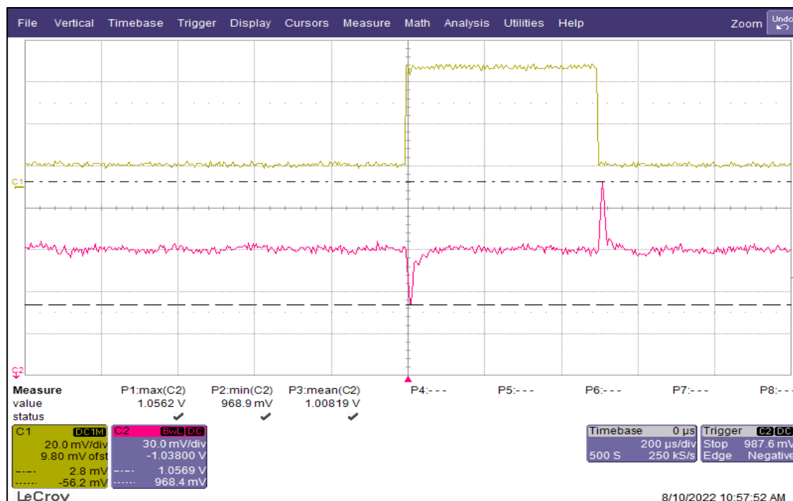
Figure 11a. Shows uncompensated s/m with C_{out}=870\mu F.
