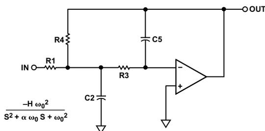
$$\frac{V_O}{V_{IN}} = \frac{-H \frac{1}{R_1 R_3 C_2 C_5}}{S^2 + S \frac{1}{C_2} \left( \frac{1}{R_1} + \frac{1}{R_3} + \frac{1}{R_4} \right) + \frac{1}{R_3 R_4 C_2 C_5}}$$
