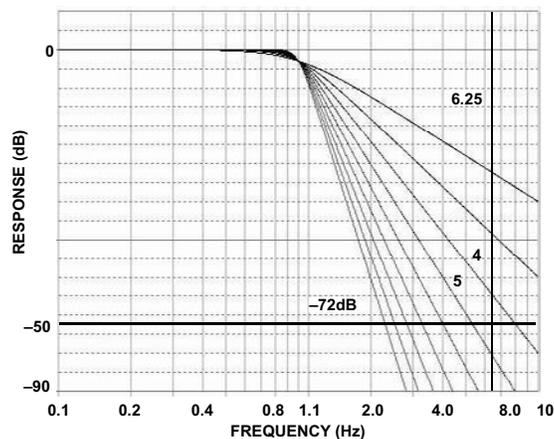
Figure 24. Determining Filter Order
