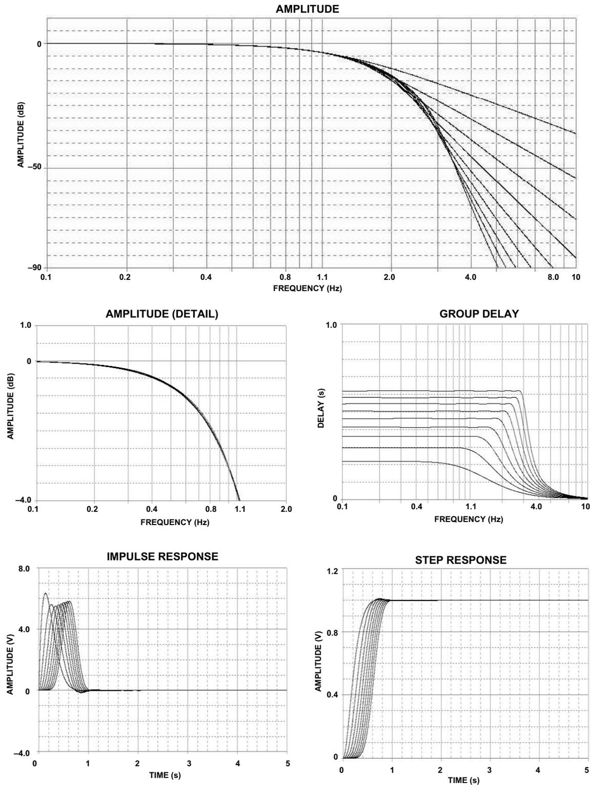
Figure 8. Linear Phase with Equiripple Error of  $0.05^\circ$  Response
