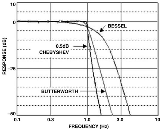
Figure 12. Amplitude Response Comparison
