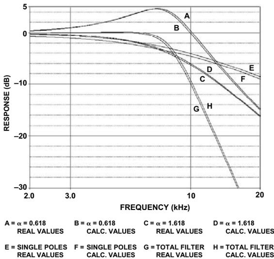
Figure 30 shows the change in the filter response due to using standard values versus exact values. Whether this is acceptable is a decision that the designer must make.
