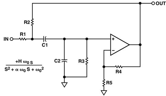
$$\frac{V_O}{V_{IN}} = \frac{H s \frac{1}{R_1 C_2}}{s^2 + s \left[ \frac{\frac{C_1}{R_3} + \frac{(C_1 + C_2)}{R_1} + \frac{C_2}{R_2} + \frac{C_1}{R_2} (1-H)}{C_1 C_2} \right] + \frac{1}{R_3 C_1 C_2} \left( \frac{R_1 + R_2}{R_1 R_2} \right)}$$
