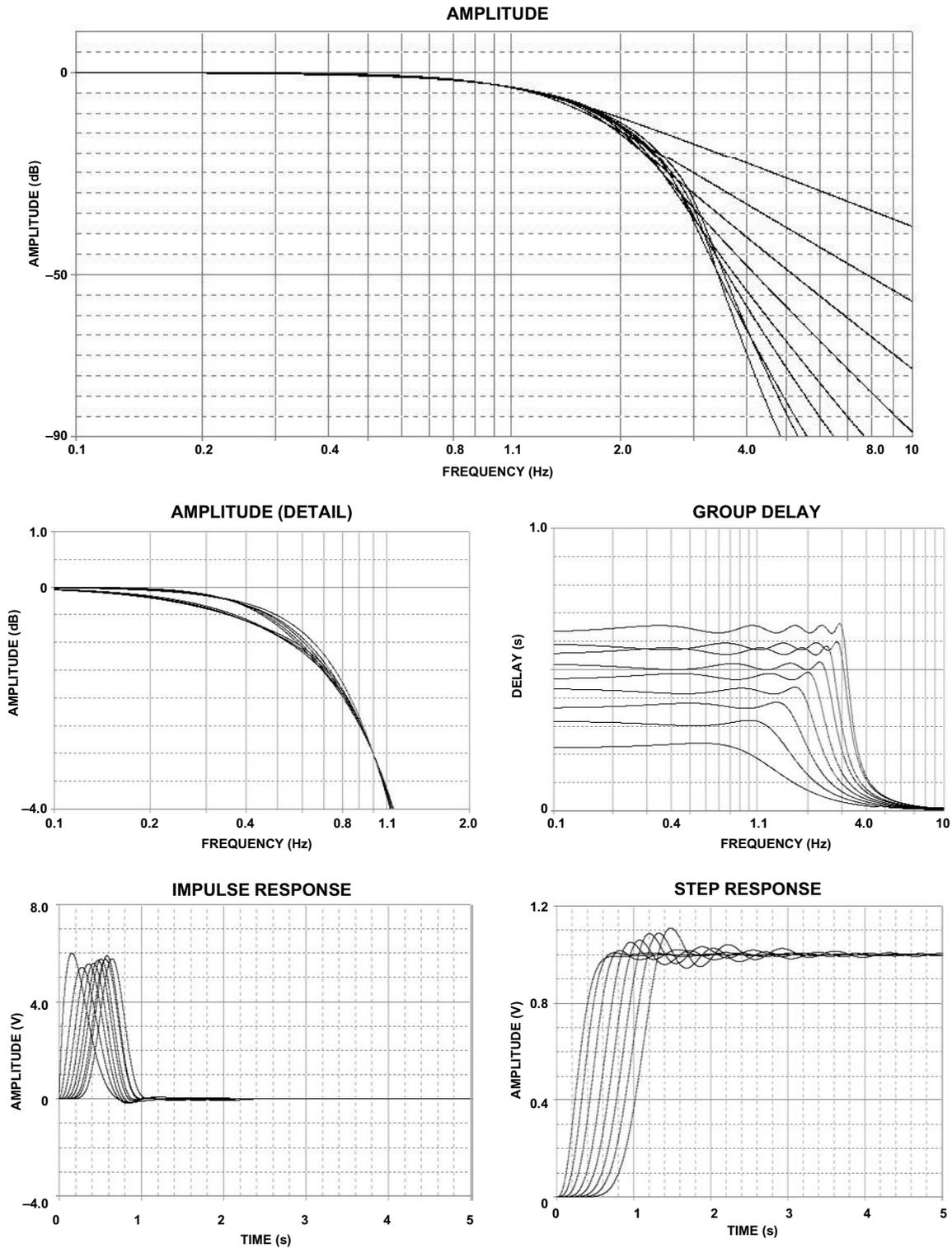
Figure 9. Linear Phase with Equiripple Error of  $0.5^\circ$  Response
