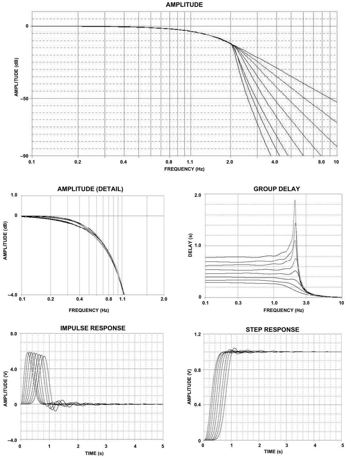
Figure 10. Gaussian-to-12 dB Response
