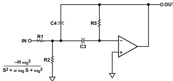
$$\frac{V_O}{V_{IN}} = \frac{-S \frac{1}{R_1 C_4}}{S^2 + S \frac{(C_3 + C_4)}{C_3 C_4 R_5} + \frac{1}{R_5 C_3 C_4} \left( \frac{1}{R_1} + \frac{1}{R_2} \right)}$$
