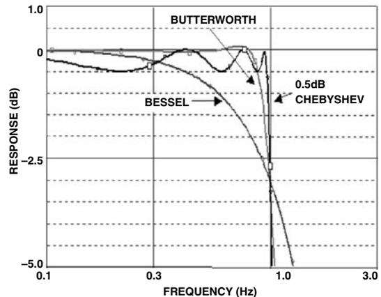
Figure 13. Amplitude Response Comparison (Detail)
