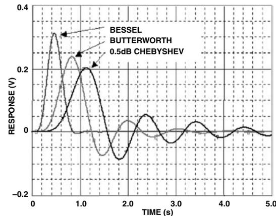
Figure 14. Impulse Response Comparison
