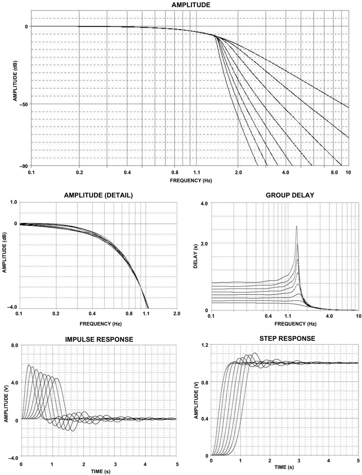
Figure 11. Gaussian-to-6 dB Response
