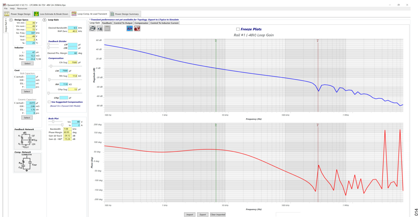
Figure 14. LTpowerCAD Setup for the LTC3896 (Third Tab Features Compensation)
