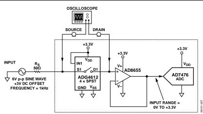
Figure 7. Single Supply Fault Protected Data Acquisition Signal Chain Circuit (Simplified Schematic: All Connections and Decoupling Not Shown)
