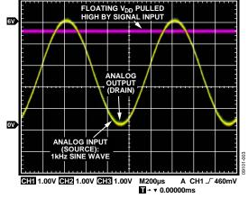
Figure 3. Standard Analog Switch with No Power Supply
