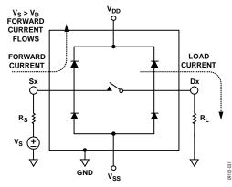
Figure 2. ESD Protection on Standard Analog CMOS Switches
