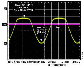
Figure 4. Standard Analog Switch with Overvoltage Condition
