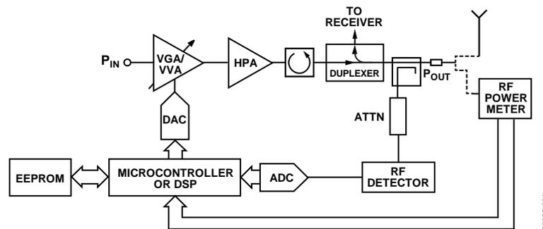
Figure 1. Typical RF Power Amplifier with Integrated Transmit Power Control
