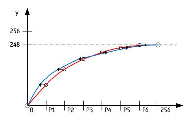
Figure 1.2 Modifying the wave for evenly distributed microsteps (example)
