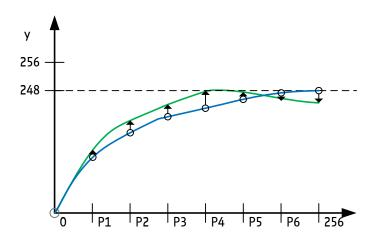
Figure 1.4 Modifying the wave for constant torque (example)
