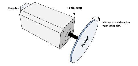
Figure 1.3 Setup for torque optimization
