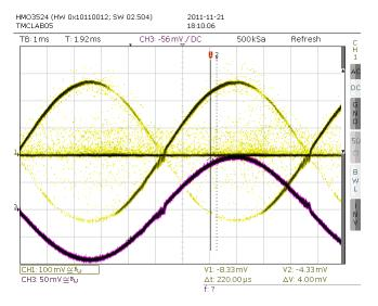
Figure 2.3 Distortion caused by too low blank time setting TBL
