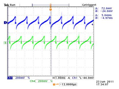
Figure 3.4 High Speed Fullstepping with Slow Decay only
