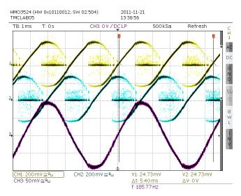
Figure 2.2 Velocity too high - motor current cannot follow
