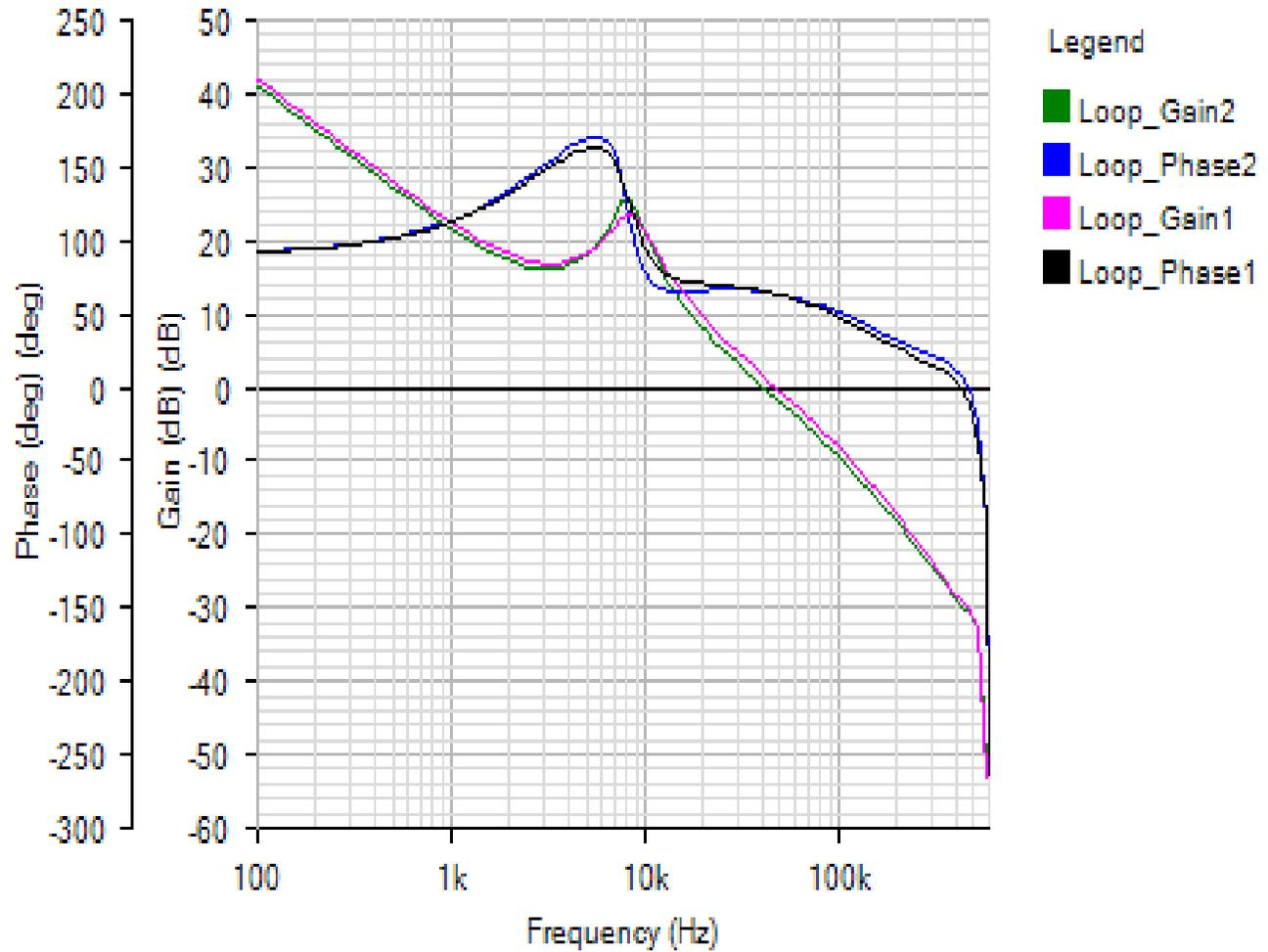
Phase Margin (output #1): 63.7° at a crossover frequency of 47.7kHz
