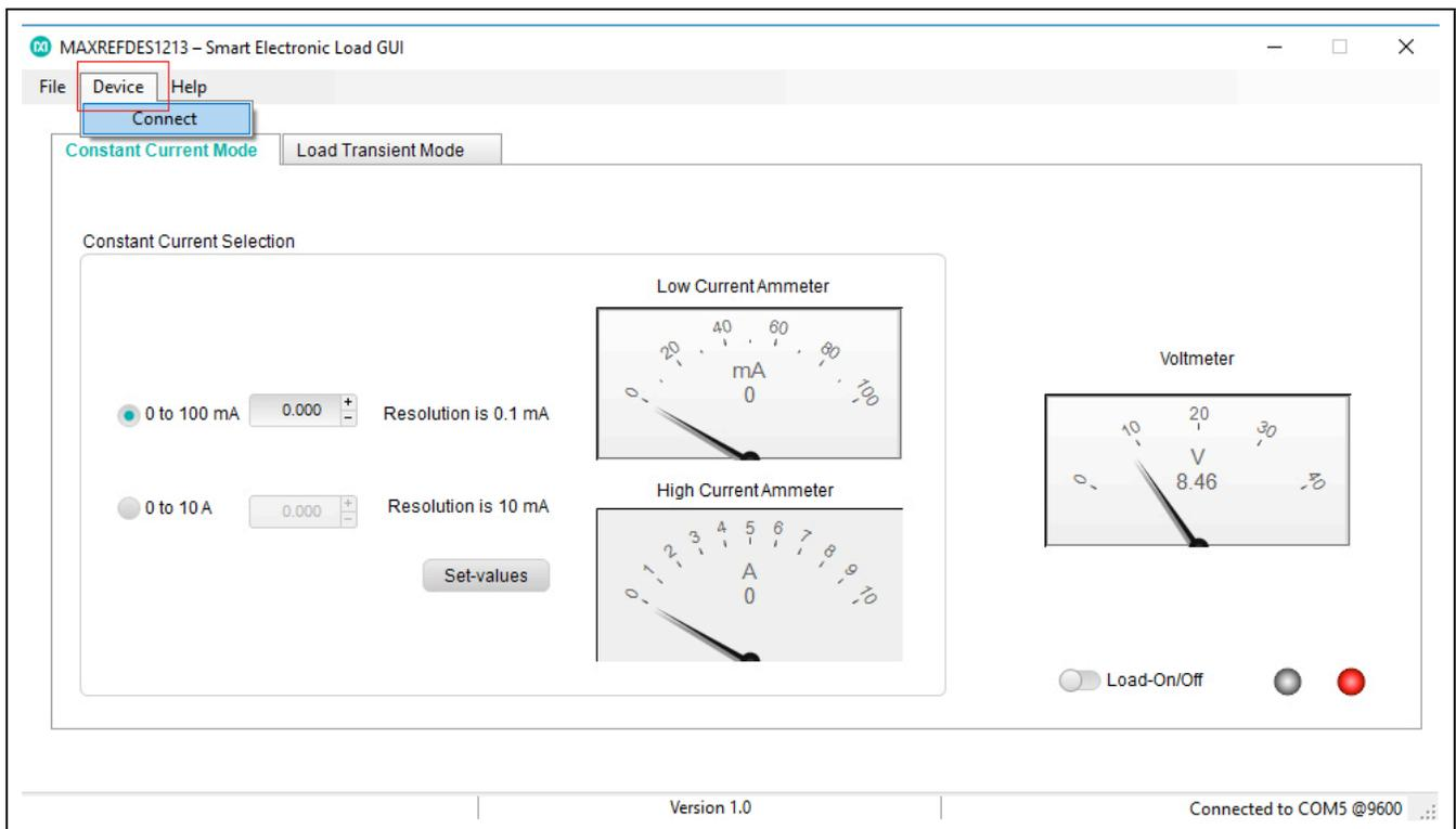
Figure 11. The Device menu option for connecting/reconnecting the GUI to the E-load.
