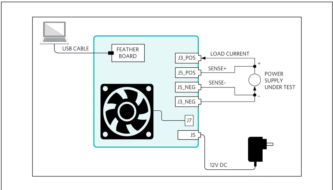
Figure 2. E-load functional diagram.
