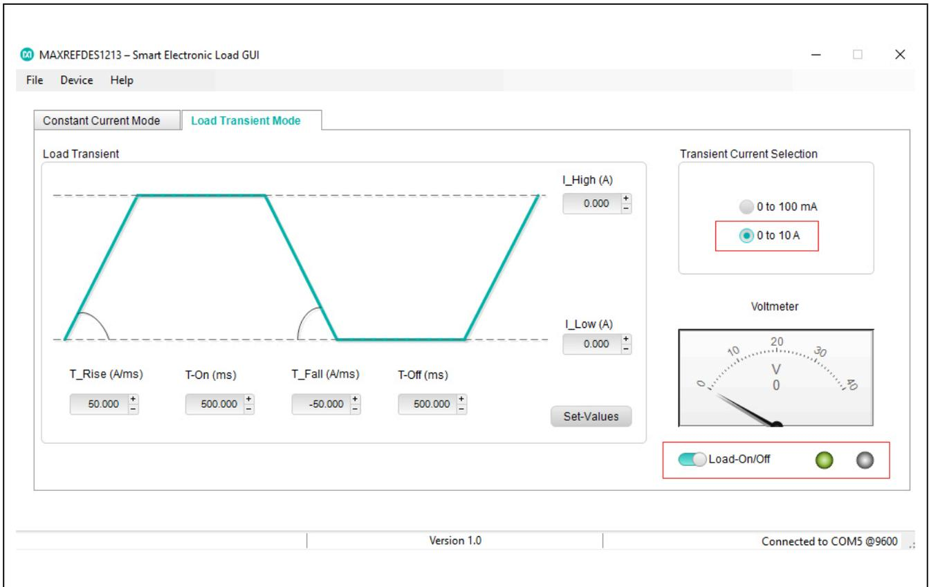
Figure 10. Load Transient Mode tab with load turned on.
