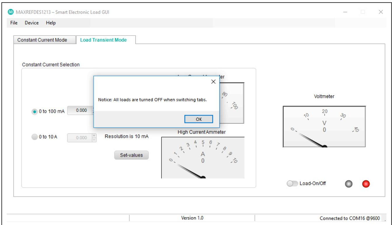
Figure 8. Switching tabs turns all loads off.
