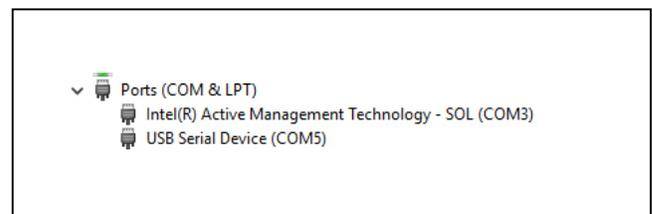
Figure 3. List of COM ports in Device Manager.
