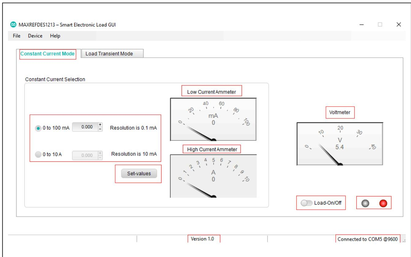
Figure 6. Constant Current Mode tab with the load turned off, and the indicator stays red.
