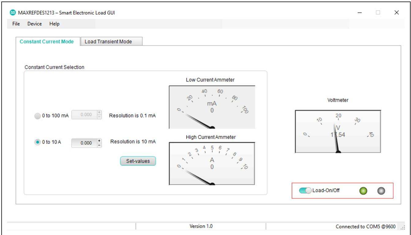
Figure 7. Constant Current Mode tab with the load turned on and the indicator turned green.
