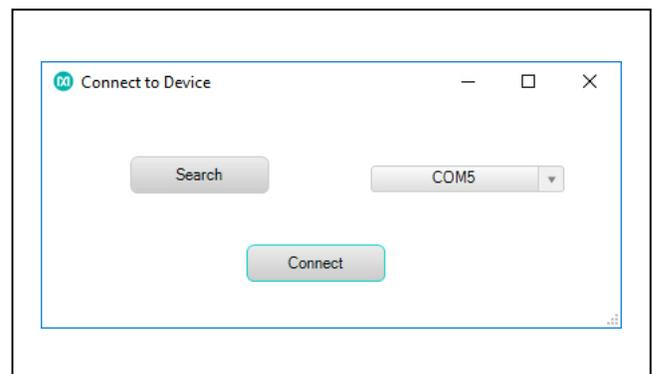
Figure 5. Select COM port 5 from the drop-down list.
