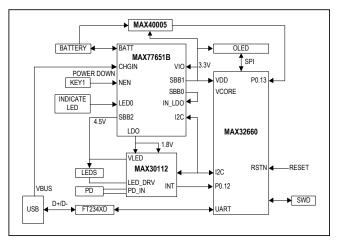
Figure 2. MAXREFDES1207 block diagram.
