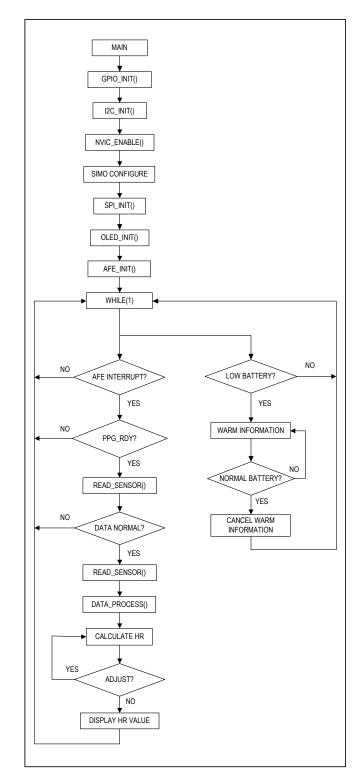
Figure 3. Main function flowchart.
