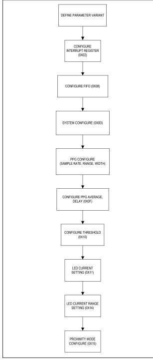
Figure 4. MAX30112 configure flowchart.
