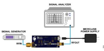
Figure 14. Phase Noise Measurement Setup
