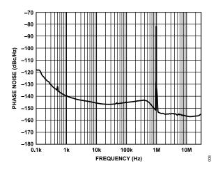
Figure 6. Phase Noise vs. Frequency Offset (433.92 MHz Input)
