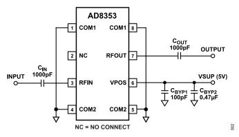
Figure 2. AD8353 Connection Diagram
