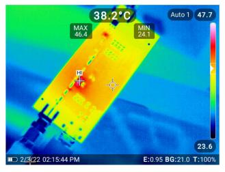
Figure 10. CN0551 Thermal Performance (RF Input Power = -10 dBm)
