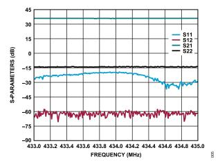
Figure 5. S-Parameters vs. Frequency
