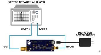
Figure 13. S-Parameter Measurement Setup
