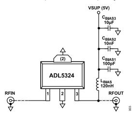
Figure 3. ADL5324 DC Bias Inductor and Capacitors
