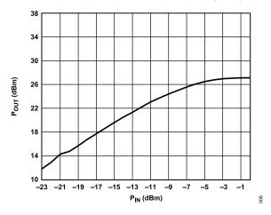
Figure 8. POUT vs. PIN (433.92 MHz Input)
