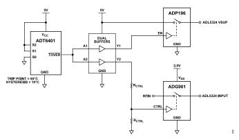
Figure 9. CN0551 Overtemperature Management Circuit
