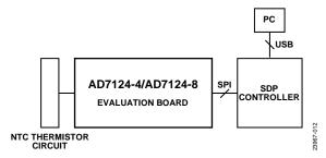
Figure 12. Test Setup Functional Diagram
