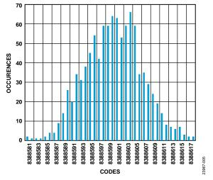
Figure 5. Histogram of Codes for a NTC Thermistor at a Temperature of 25°C, Post Filter in Low Power Mode, 25 SPS
