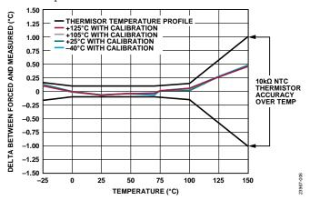
Figure 6. Thermistor Temperature Accuracy Measurement, Sinc<sup>4</sup> Filter, Full Power Mode, 50 SPS
