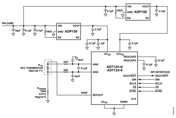
Figure 1. Thermistor Measurement Block Diagram
