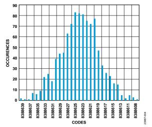
Figure 4. Histogram of Codes for a NTC Thermistor at a Temperature of 25 ℃ with a Sinc<sup>4</sup> Filter in Full Power Mode, 50 SPS
