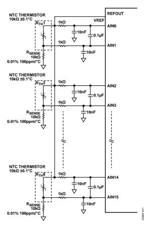
Figure 11. 10 k $\Omega$  NTC Thermistor Multiple Analog Input Configuration Using the AD7124-8
