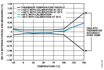
Figure 9. Thermistor Temperature Accuracy Measurement, Post Filter, Low Power Mode, 25 SPS at Ambient
