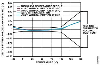
Figure 8. Thermistor Temperature Accuracy Measurement, Sinc<sup>4</sup> Filter, Full Power Mode, 50 SPS at Ambient
