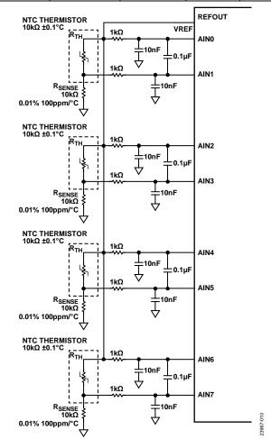
Figure 10. 10 k $\Omega$  NTC Thermistor Multiple Analog Input Configuration Using the AD7124-4
