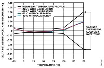
Figure 7. Thermistor Temperature Accuracy Measurement, Post Filter, Low Power Mode, 25 SPS
