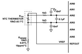
Figure 3. 10 k $\Omega$  NTC Thermistor Analog Input Configuration
