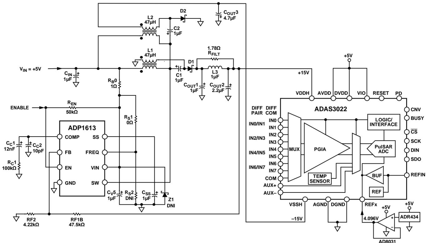
Figure 1. Complete 5 V, Single-Supply, 8-Channel Data Acquisition Solution with Integrated PGA (Simplified Schematic: All Connections and Decoupling Not Shown)
