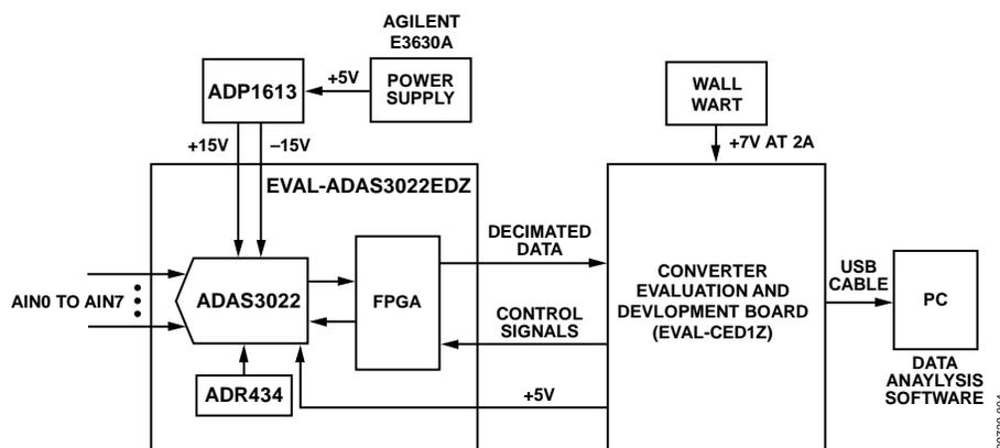
Figure 4. Test Setup Functional Block Diagram
