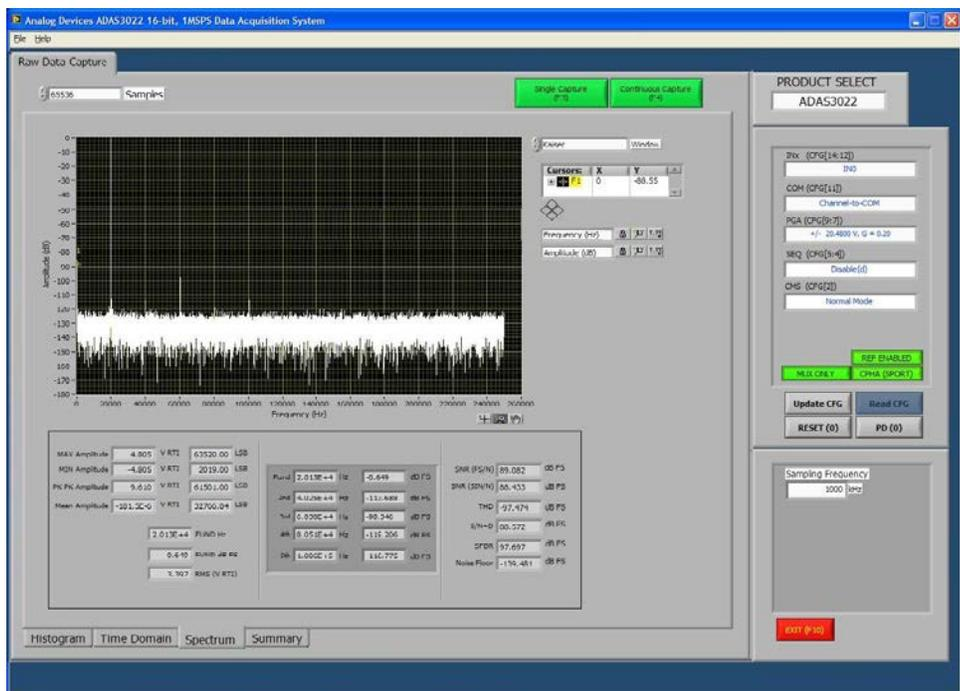
Figure 3. FFT Output of the [ADAS3022](#) Using the [EVAL-CED1Z](#) Evaluation Board and Software
