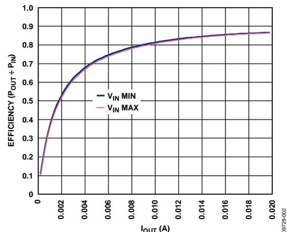
Figure 2. [ADP1613](#) Efficiency ( $P_{OUT}/P_{IN}$ ) vs. Output Current ( $I_{OUT}$ )
