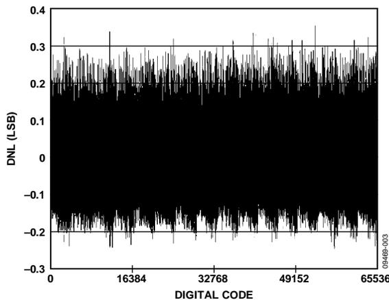
Figure 3. Differential Nonlinearity (DNL) Measurement
