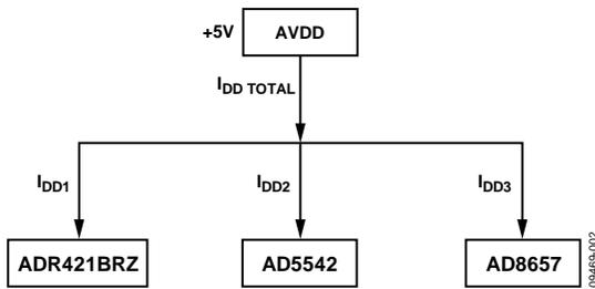
Figure 2. Power Supply Current Measurements
