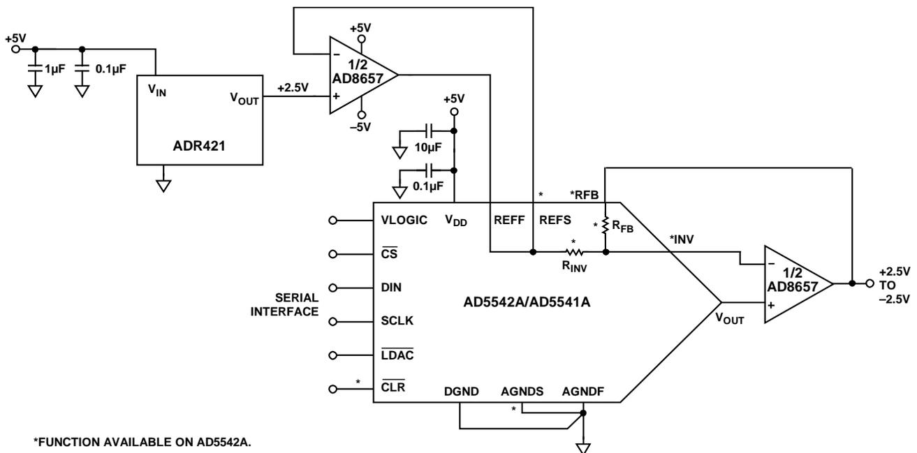
Figure 1. Precision DAC Configuration (Simplified Schematic: All Connections and Decoupling Not Shown)
