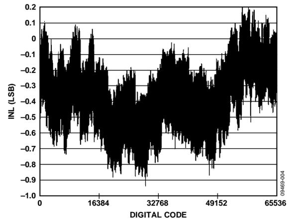
Figure 4. Integral Nonlinearity (INL) Measurement
