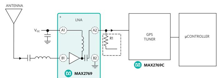
Figure 2. GPS Receiver Front-End Circuitry
