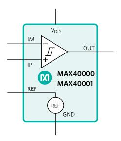
Figure 5. MAX40000/MAX40001 Functional Diagram
