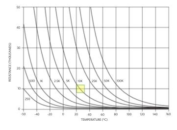
Figure 4. Resistance-Temperature Curves for Nine Common Thermistors
