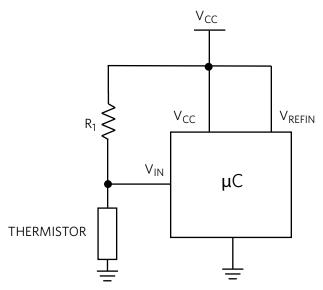
Figure 2. Temperature Monitoring Circuit Using a Thermistor
