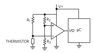
Figure 3. Temperature Monitoring Using a Comparator
