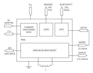
Figure 2. Highly Integrated SIMO PMIC Block Diagram
