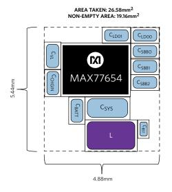
Figure 6. SIMO PMIC Solution with Minimal Board Space (19.2mm<sup>2</sup>)
