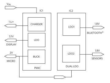
Figure 8. Typical Wearable Power Flow Diagram
