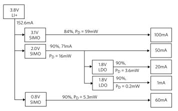
Figure 3. Power Tree of a High-Efficiency SIMO
