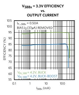
Figure 7. Buck vs. Buck-Boost Efficiency
