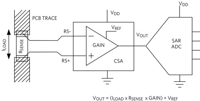
Figure 4. CSA with a Kelvin-Sensing PCB Resistor
