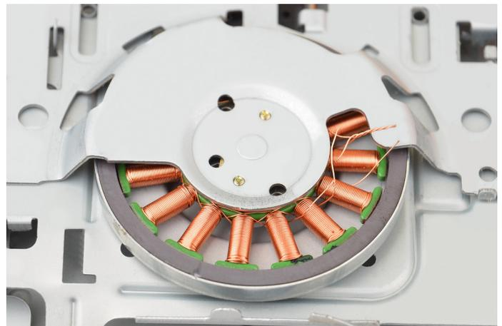
*Figure 2. BLDC with Removed Upper Cover and Magnet Rotor*
