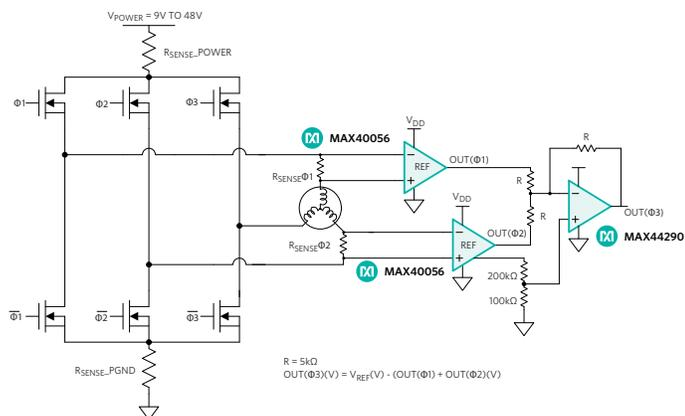
Figure 7. Economic Current Sensing in a 3-Phase Servo Motor by Sensing Two Phases
