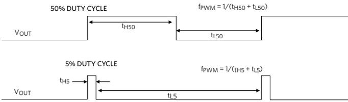
Figure 3. PWM Voltage Signal ( $V_{OUT}$ ) with a 50% and 5% Duty Cycle
