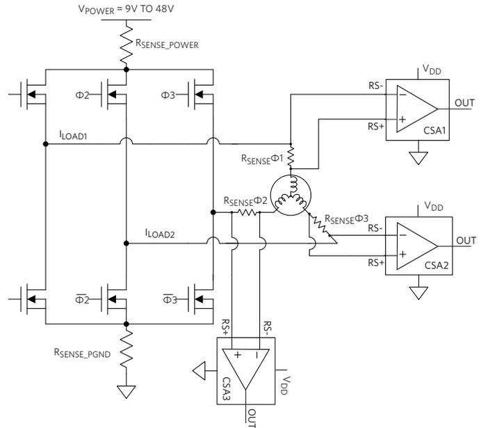
Figure 5. Current Sensing in a 3-Phase Servo Motor
