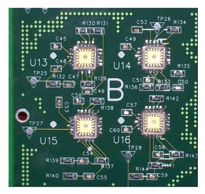
Figure 4.1. Single event test board mounted on the test stage at Berkeley. The board has four units-under-test mounted simultaneously to minimize vacuum breaks during testing. There is also a heater plate mounted to the backside of the board to provide the elevated temperature required for this testing.
