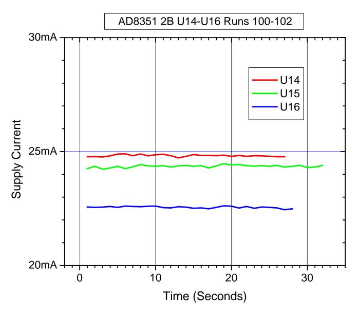
Figure 5.1. Supply current on  $+V_S$  and  $-V_S$  versus time for AD8351 unit-under-test number U14, U15 and U16. The testing was performed at an effective LET of  $83 \text{MeV-cm}^2/\text{mg}$  using Xe at an energy of 10 MeV/n. As seen in the figure, the supply current shows no significant increase during the run, indicating that the unit-under-test has not experienced a latch-up event.
