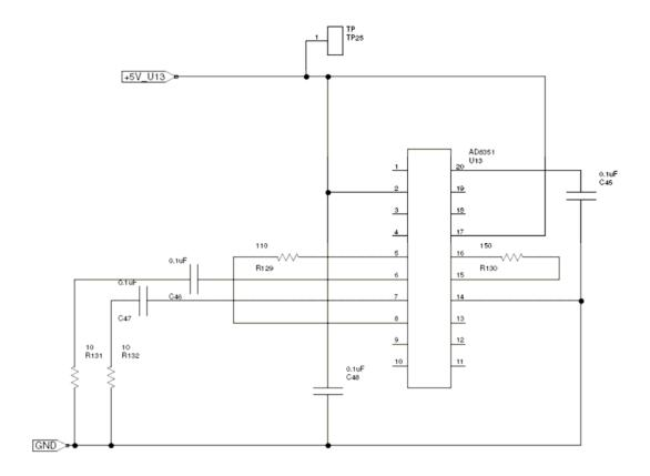
Figure B.1. Schematic drawing of the bias configuration used for the SEL test described in this final report.
