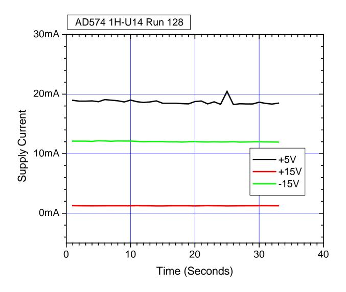
Figure 5.2. Supply current on versus time for AD574 unit numbers U14. The testing was performed at an effective LET of 83MeV-cm²/mg using Xe at an energy of 10MeV/n. As seen in the figure, the supply current shows no significant increase during the run, indicating that the units-under-test have not experienced a latch-up event.
