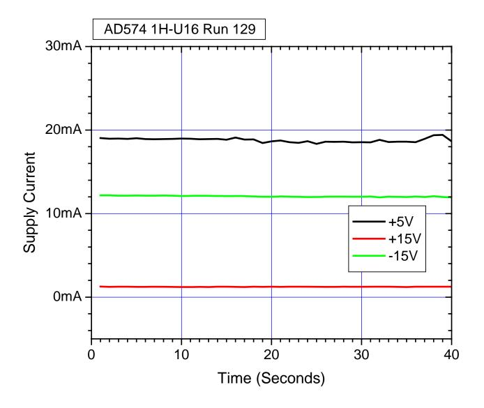
Figure 5.3. Supply current on versus time for AD574 unit numbers U16. The testing was performed at an effective LET of 83MeV-cm²/mg using Xe at an energy of 10MeV/n. As seen in the figure, the supply current shows no significant increase during the run, indicating that the units-under-test have not experienced a latch-up event.
