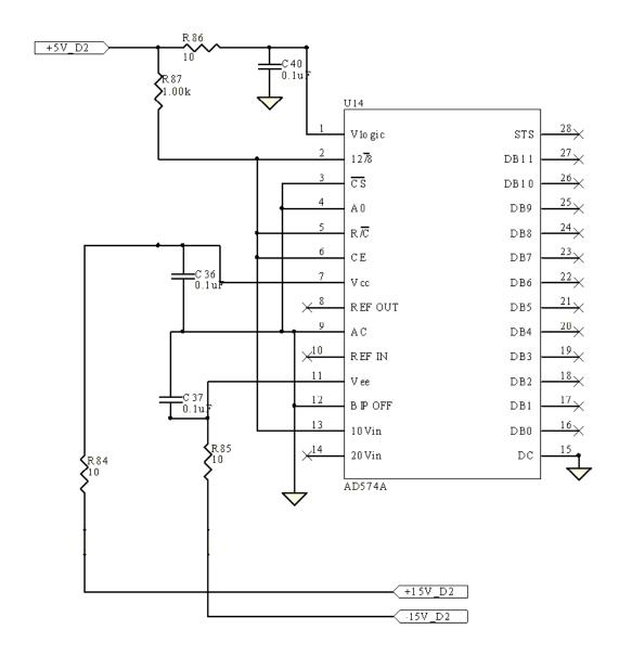
Figure B.1. Schematic drawing of the configurations used for the SEL test described in this final report.
