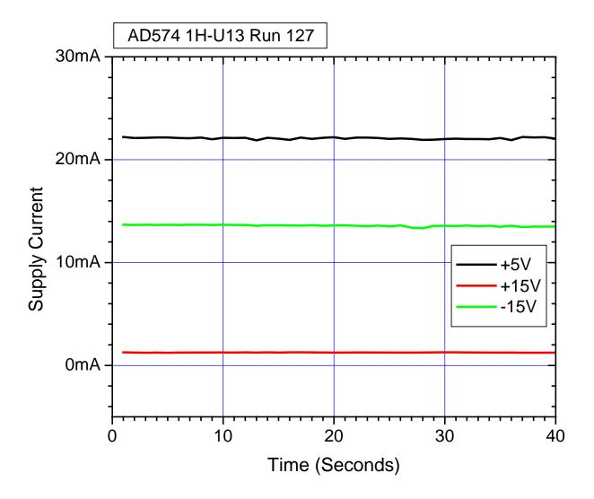
Figure 5.1. Supply current on versus time for AD574 unit numbers U13. The testing was performed at an effective LET of 83MeV-cm²/mg using Xe at an energy of 10MeV/n. As seen in the figure, the supply current shows no significant increase during the run, indicating that the units-under-test have not experienced a latch-up event.
