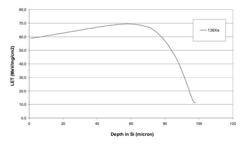
Figure 3.1. Range of the 10 MeV/n Xe beam into silicon. The range to the Bragg Peak is approximately  $60 \mu \text{m}$  while the surface LET is approximately 58 MeV-cm2/mg.
