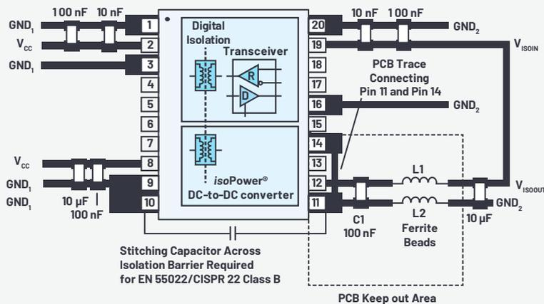
Figure 1. PCB decoupling for 2-layer and 4-layer PCB.
