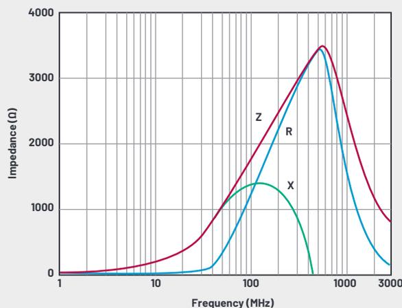
Figure 4. BLM15HD182SN1 impedance curve.
