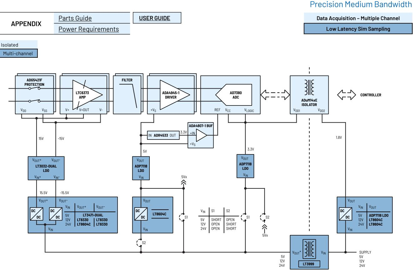
\*The actual output voltage of LT3999 isolated converter depends primarily on the turns ratio of the transformer used. See LT3999 datasheet for details.
