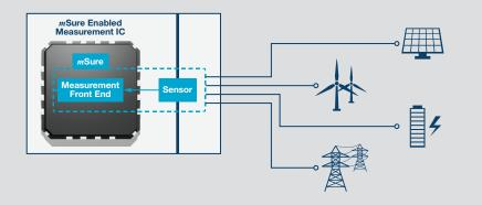
*m*Sure is an exciting and innovative technology that resides in energy measurement ICs and provides a comprehensive accuracy monitoring and self diagnostic capability for the entire system, including the sensor.
