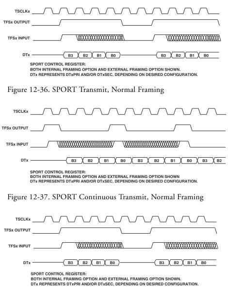
Figure 12-38. SPORT Transmit, Alternate Framing
