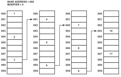
THE COLUMNS ABOVE SHOW THE SEQUENCE IN ORDER OF LOCATIONS ACCESSED IN ONE PASS. THE SEQUENCE REPEATS ON SUBSEQUENT PASSES.
