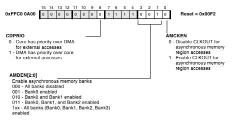
Figure 18-3. Asynchronous Memory Global Control Register
