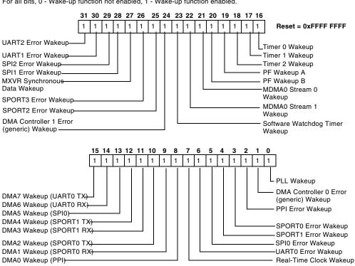
System Interrupt Wakeup-Enable Register 0 (SIC\_IWR0)
