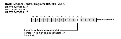
Figure 13-3. UART Modem Control Register
