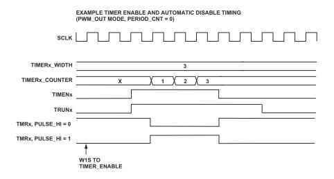
Figure 16-11. Timer Enable and Automatic Disable Timing
