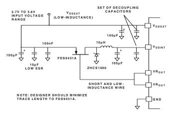
Figure 8-7. Processor Voltage Regulator
