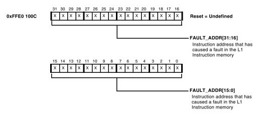
Figure 6-25. ICPLB Fault Address Register
