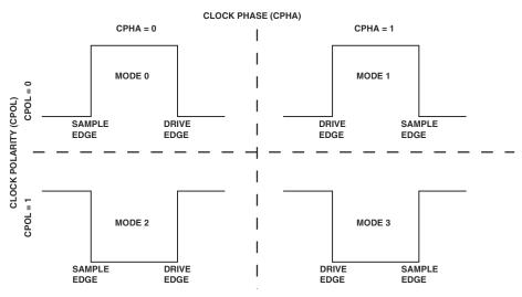
Figure 10-11. SPI Modes of Operation
