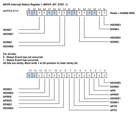
Figure 21-9. MXVR Interrupt Status Register\_1 (MXVR\_INT\_STAT\_1)
