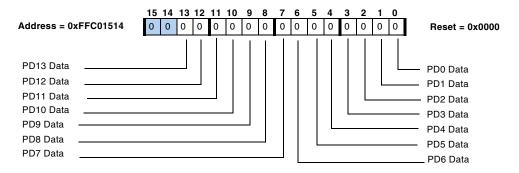
Figure 15-11. GPIO Port D Data Register
