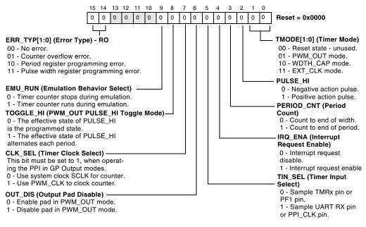
Figure 1. Register Diagram Example
