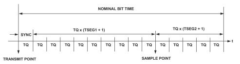
Figure 19-7. Three Phases of a CAN Bit
