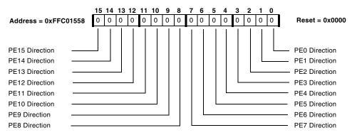
Figure 15-6. GPIO Port E Direction Register
