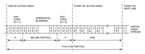
Figure 11-6. ITU-R 656 8-Bit Parallel Data Stream for NTSC (PAL) Systems
