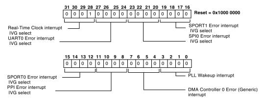
Figure 4-12. System Interrupt Assignment Register 0 (SIC\_IAR0)
