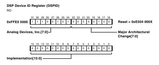
Figure 23-15. DSP Device ID Register
