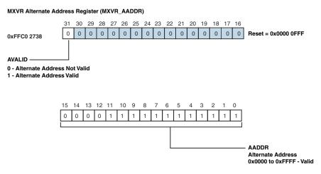
Figure 21-18. MXVR Alternate Address Register (MXVR\_AADDR)
