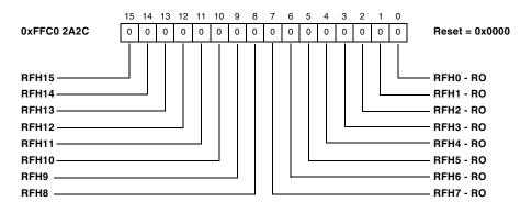
Figure 19-50. Remote Frame Handling Register 1
