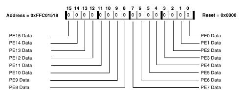
Figure 15-12. GPIO Port E Data Register
