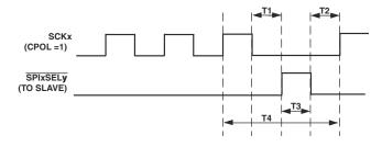
Figure 10-14. SPI Timing
