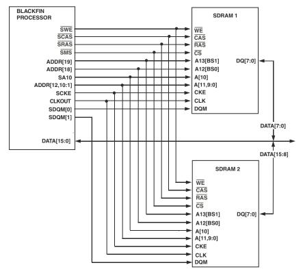
Figure 18-11. 16M byte SDRAM System Example
