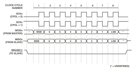
Figure 10-12. SPI Transfer Protocol for CPHA = 0
