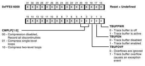
Figure 23-9. Trace Buffer Control Register
