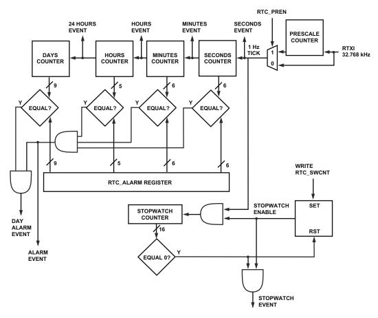
Figure 17-1. RTC Block Diagram
