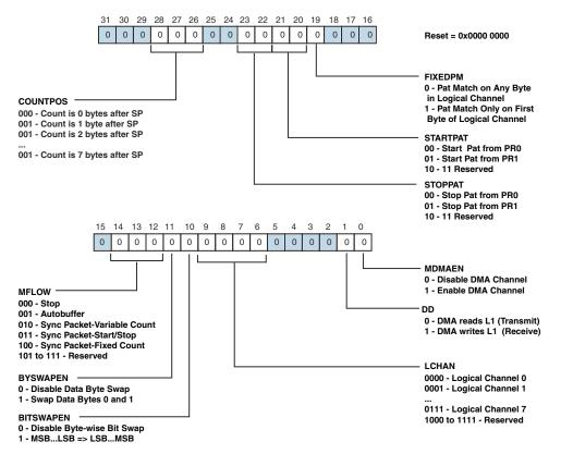
Figure 21-21. MXVR DMA Channel x Configuration Register (MXVR\_DMAx\_CONFIG)
