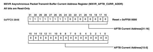
Figure 21-30. MXVR Asynchronous Packet Transmit Buffer Current Address Register (MXVR\_APTB\_CURR\_ADDR)
