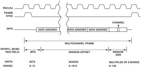
NOTE: FRAME LENGTH IS SET BY FRAME SYNC DIVIDE OR EXTERNAL FRAME SYNC PERIOD.
