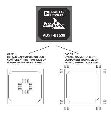
Figure 22-5. Bypass Capacitor Placement
