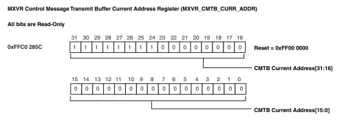
Figure 21-35. MXVR Control Message Transmit Buffer Current Address Register (MXVR\_CMTB\_CURR\_ADDR)
