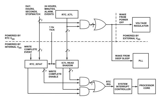
Figure 17-3. RTC Interrupt Structure
