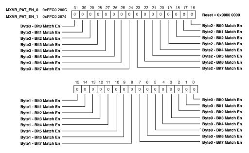
Figure 21-39. MXVR Pattern Enable Registers (MXVR\_PAT\_EN\_0, MXVR\_PAT\_EN\_1)
