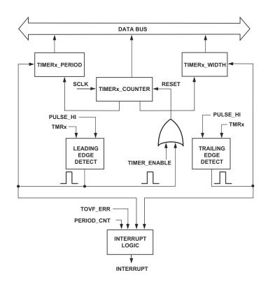
Figure 16-16. Timer Flow Diagram, WDTH\_CAP Mode
