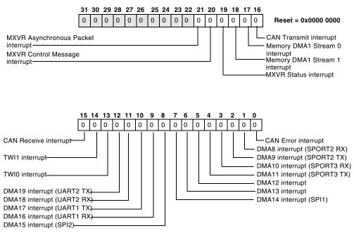
Figure 4-11. System Interrupt Mask Register 1 (SIC\_IMASK1)
