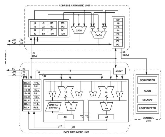
Figure 2-1. Processor Core Architecture
