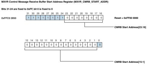
Figure 21-32. MXVR Control Message Receive Buffer Start Address Register (MXVR\_CMRB\_START\_ADDR)
