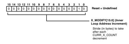
Figure 9-5. Inner Loop Address Increment Register
