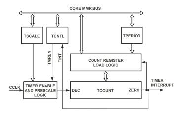
Figure 16-25 provides a block diagram of the Core timer.
