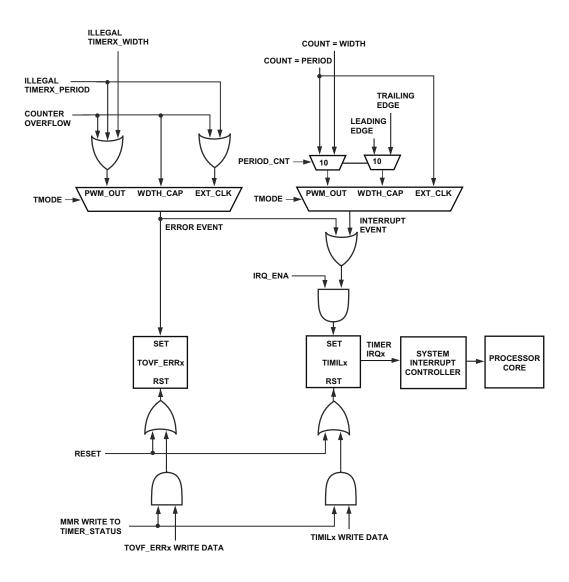
Figure 16-24. Timers Interrupt Structure
