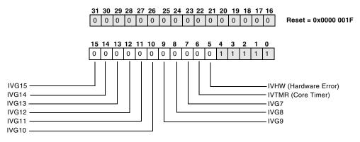
Figure 4-19. Core Interrupt Mask Register
