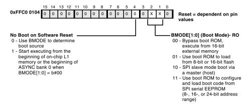
Figure 3-2. System Reset Configuration Register
