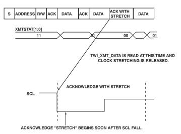
Figure 20-27. Clock Stretching During FIFO Underflow
