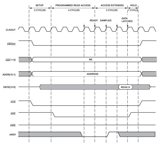
Figure 18-10. Inserting Wait States Using ARDY
