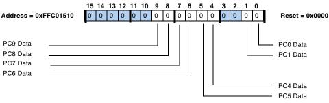
PC1 and PC4 are 5V-tolerant input/open-drain output pins.
