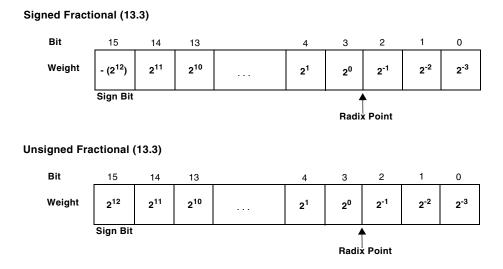
Figure D-2. Example of Fractional Format
