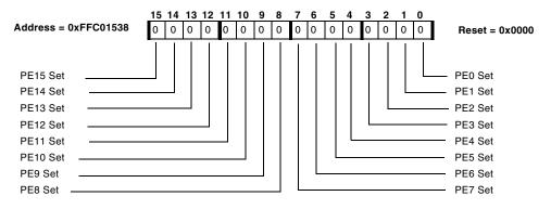
Figure 15-18. GPIO Port E Set Register
