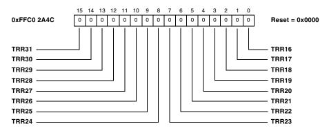
Figure 19-44. Transmission Request Reset Register 2
