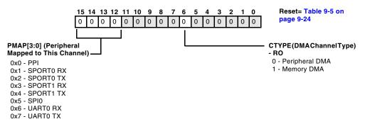
Figure 9-12. DMA Controller 0 Peripheral Map Register
