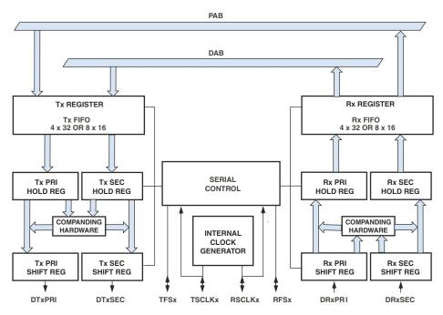
NOTE 1: ALL WIDE ARROW DATA PATHS ARE 16 OR 32 BITS WIDE, DEPENDING ON SLEN. FOR SLEN = 2 TO 15, A 16-BIT DATA PATH WITH 8-DEEP FIFO IS USED. FOR SLEN = 16 TO 31, A 32-BIT DATA PATH WITH 4-DEEP FIFO IS USED. NOTE 2: TX REGISTER IS THE BOTTOM OF THE TX FIFO, RX REGISTER IS THE TOP OF THE RX FIFO.
