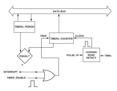
Figure 16-23. Timer Flow Diagram, EXT\_CLK Mode
