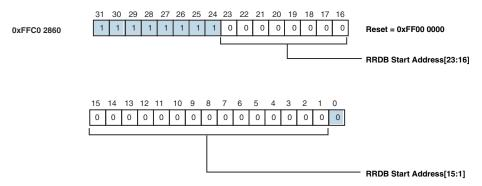
Figure 21-36. MXVR Remote Read Buffer Start Address Register (MXVR\_RRDB\_START\_ADDR)
