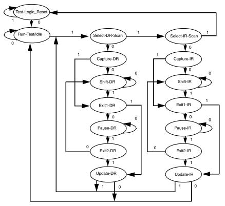
Figure C-1. TAP Controller State Diagram
