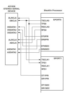
Figure 12-3. Stereo Serial Connection
