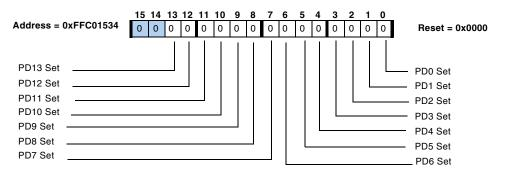
Figure 15-17. GPIO Port D Set Register
