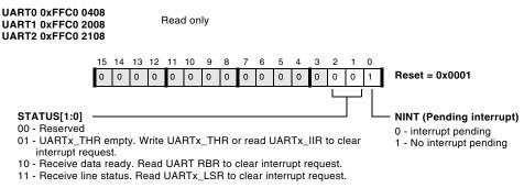
Figure 13-8. UART Interrupt Identification Register
