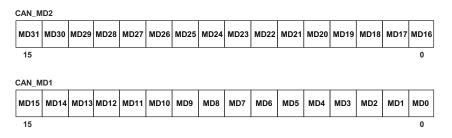
Figure 19-4. CAN Register Pairs
