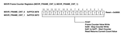
Figure 21-40. MXVR Frame Counter Registers (MXVR\_FRAME\_CNT\_0, MXVR\_FRAME\_CNT\_1)
