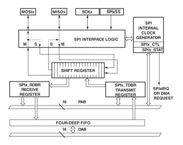
Figure 10-1. SPI Block Diagram
