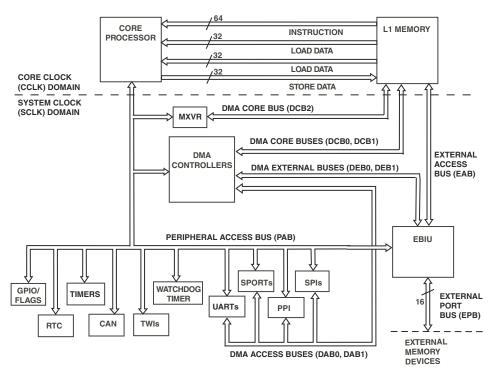
Figure 6-2. Processor Memory Architecture
