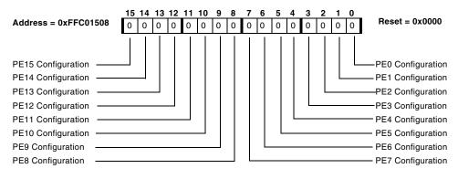
Figure 15-3. GPIO Port E Configuration Register
