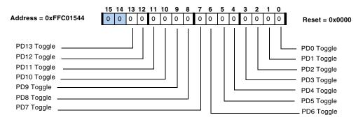
Figure 15-20. GPIO Port D Toggle Register
