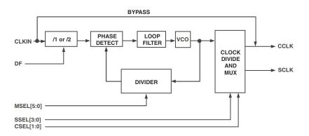
Figure 8-1. PLL Block Diagram
