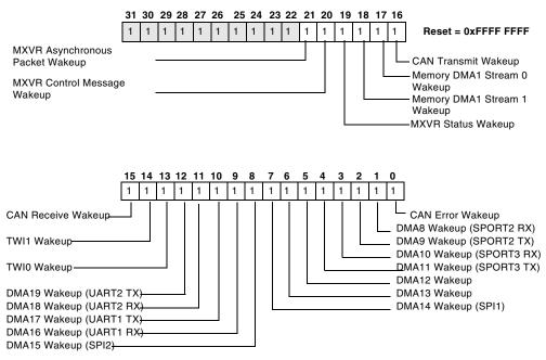
Figure 4-7. System Interrupt Wakeup-Enable Register 1 (SIC\_IWR1)
