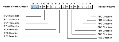
Figure 15-5. GPIO Port D Direction Register
