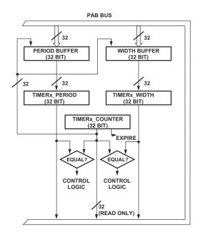
Figure 16-1. Timer Block Diagram
