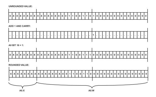
Figure 2-7. Avoiding Net Bias in Unbiased Multiplier Rounding
