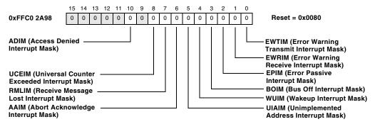
Figure 19-18. Global CAN Interrupt Mask Register
