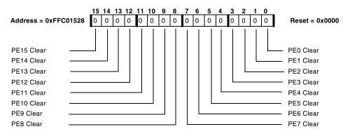
Figure 15-15. GPIO Port E Clear Register
