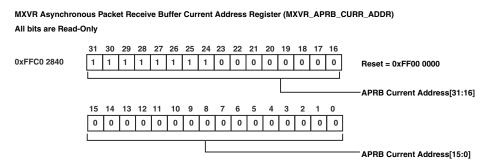
Figure 21-28. MXVR Asynchronous Packet Receive Buffer Current Address Register (MXVR\_APRB\_CURR\_ADDR)
