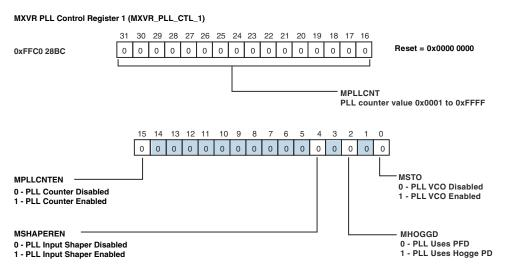
Figure 21-4. MXVR PLL Control Register 1 (MXVR\_PLL\_CTL\_1)
