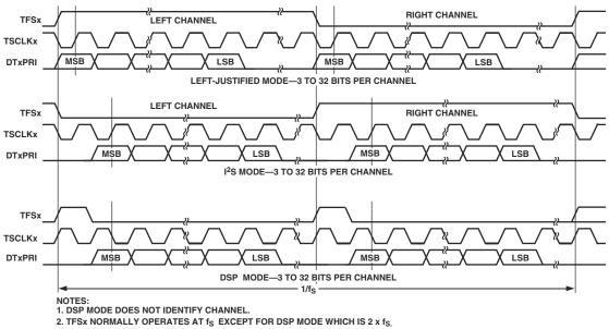
3. TSCLKx FREQUENCY IS NORMALLY 64 x TFS BUT MAY BE OPERATED IN BURST MODE.
