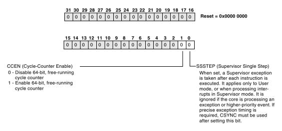
Figure 4-3. System Configuration Register
