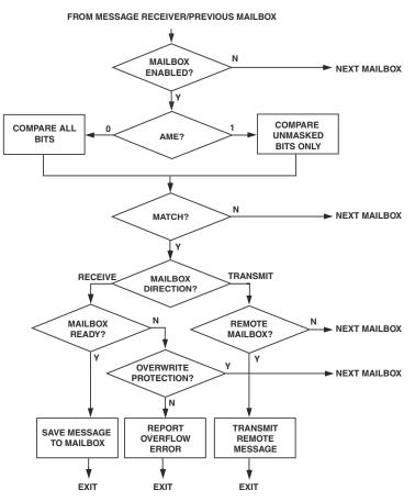
Figure 19-10. CAN Receive Operation Flow Chart
