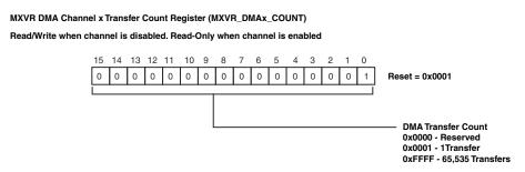
Figure 21-24. MXVR DMA Channel x Transfer Count Registers (MXVR\_DMAx\_COUNT)
