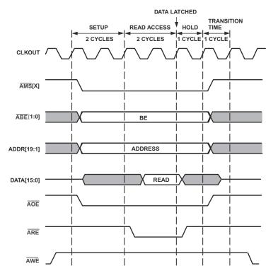
Figure 18-8. Asynchronous Read Bus Cycles
