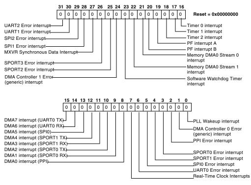
Figure 4-8. System Interrupt Status Register 0 (SIC\_ISR0)
