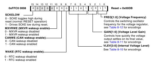
Figure 8-8. Voltage Regulator Control Register
