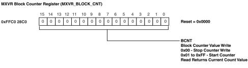
Figure 21-42. MXVR Block Counter Register (MXVR\_BLOCK\_CNT)
