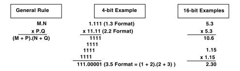
Figure D-3. Format of Multiplier Result
