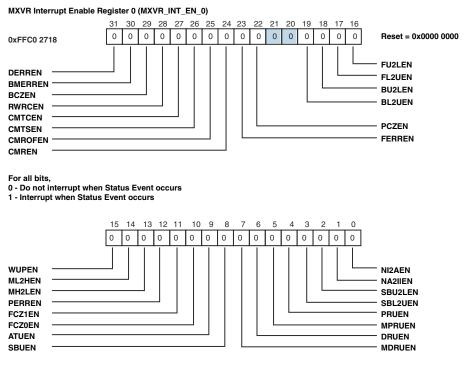
Figure 21-10. MXVR Interrupt Enable Register 0 (MXVR\_INT\_EN\_0)
