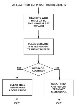
Figure 19-8. CAN Transmit Operation Flow Chart
