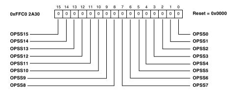
Overwrite Protection/Single Shot Transmission Register 1 (CAN\_OPSS1)
