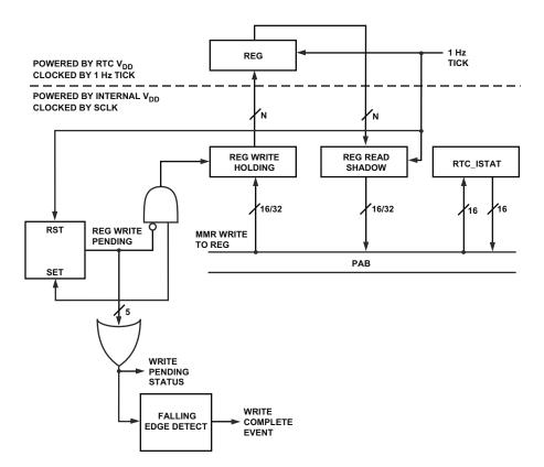
Figure 17-2. RTC Register Architecture
