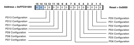
Figure 15-2. GPIO Port D Configuration Register
