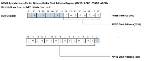
Figure 21-27. MXVR APRB Start Address Register (MXVR\_APRB\_START\_ADDR)
