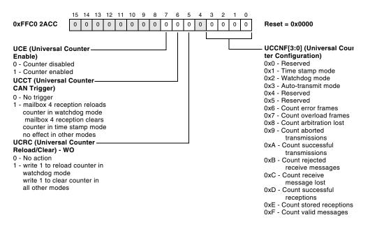
Figure 19-58. Universal Counter Configuration Mode Register
