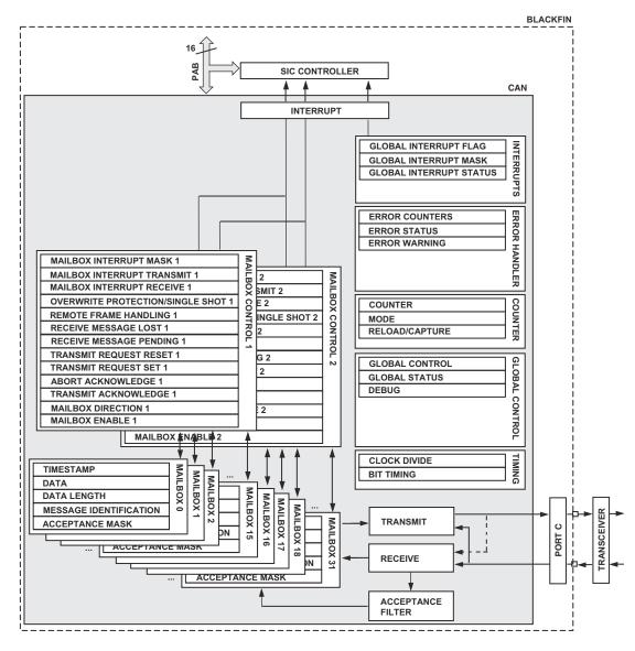
Figure 19-2. CAN Block Diagram
