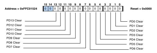
Figure 15-14. GPIO Port D Clear Register
