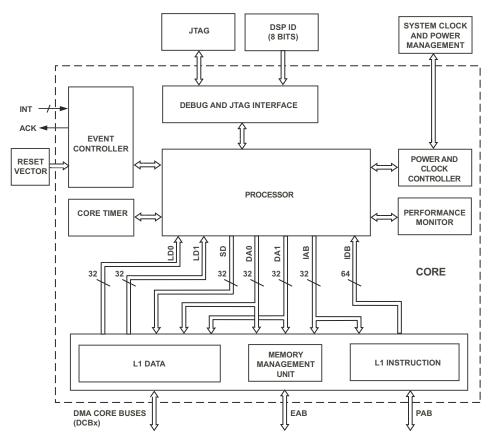
Figure 7-2. Core Block Diagram
