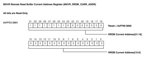
Figure 21-37. MXVR Remote Read Buffer Current Address Register (MXVR\_RRDB\_CURR\_ADDR)
