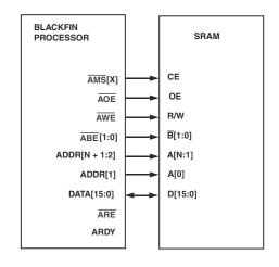
Figure 22-3. Interface to 16-bit SRAM
