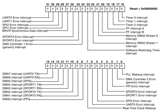
Figure 4-10. System Interrupt Mask Register 0 (SIC\_IMASK0)
