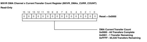
Figure 21-25. MXVR DMA Channel x Current Transfer Count Registers (MXVR\_DMAx\_CURR\_COUNT)
