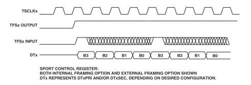
Figure 12-39. SPORT Continuous Transmit, Alternate Framing
