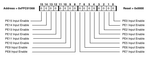
Figure 15-9. GPIO Port E Input Enable Register
