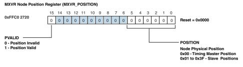
Figure 21-12. MXVR Node Position Register (MXVR\_POSITION)
