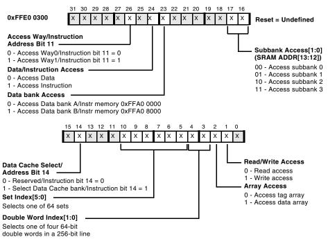
Figure 6-14. Data Test Command Register
