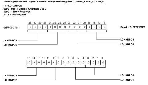
Figure 21-20. MXVR Synchronous Logical Channel Assignment Register (MXVR\_SYNC\_LCHAN\_0)
