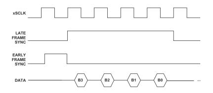
Figure 12-19. Normal Versus Alternate Framing
