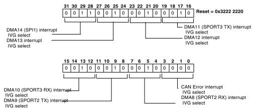
Figure 4-16. System Interrupt Assignment Register 4 (SIC\_IAR4)
