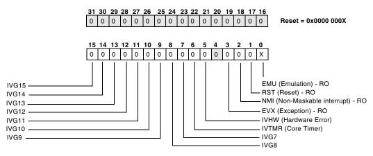
Figure 4-20. Core Interrupt Latch Register
