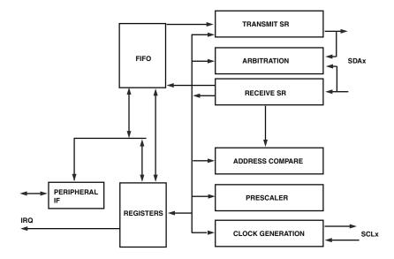
Figure 20-1. TWI Block Diagram
