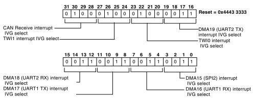
Figure 4-17. System Interrupt Assignment Register 5 (SIC\_IAR5)
