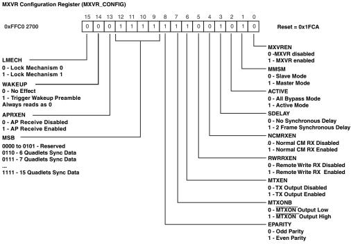
Figure 21-2. MXVR Configuration Register (MXVR\_CONFIG)
