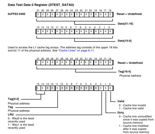
Figure 6-16. Data Test Data 0 Register
