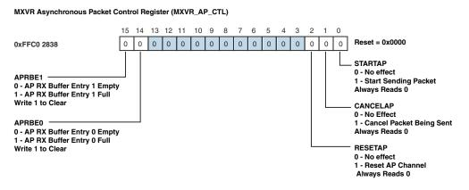
Figure 21-26. MXVR Asynchronous Packet Control Register (MXVR\_AP\_CTL)
