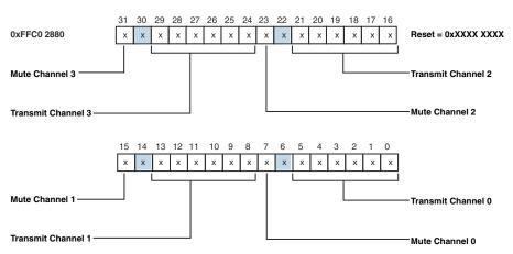
Figure 21-41. MXVR Routing Register 0 (MXVR\_ROUTING\_0)
