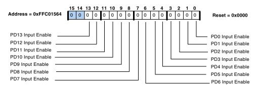
Figure 15-8. GPIO Port D Input Enable Register
