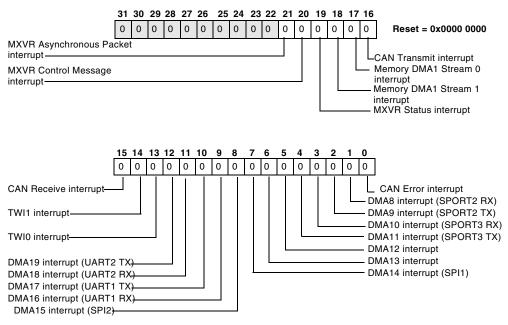
Figure 4-9. System Interrupt Status Register 1 (SIC\_ISR1)
