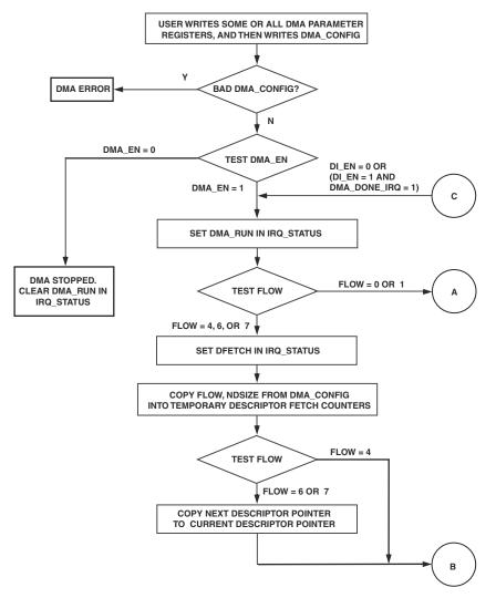
Figure 9-16. DMA Flow, from DMA Controller point of view (1 of 2)
