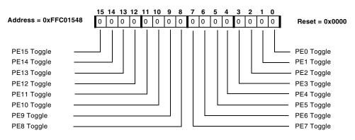
Figure 15-21. GPIO Port E Toggle Register
