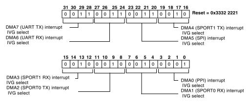
Figure 4-13. System Interrupt Assignment Register 1 (SIC\_IAR1)
