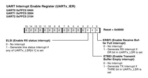
Figure 13-7. UART Interrupt Enable Register
