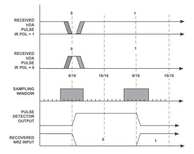
Figure 13-13. IrDA Receiver Pulse Detection
