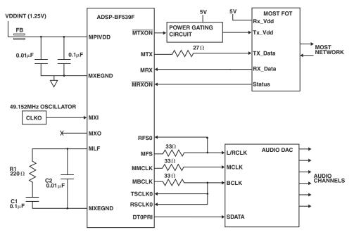
Figure 21-1. Example Connections of ADSP-BF539 to MOST Network
