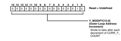
Outer Loop Address Increment Register (DMAx\_Y\_MODIFY / MDMAx\_yy\_Y\_MODIFY) R/W prior to enabling channel, RO after enabling channel
