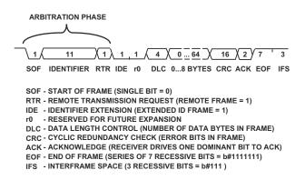
Figure 19-5. Standard CAN Frame
