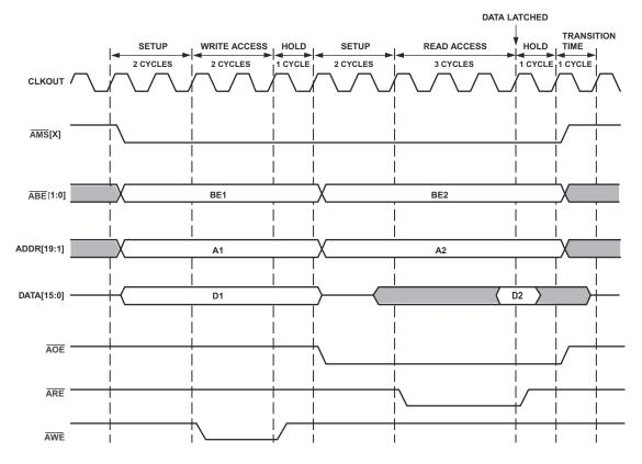
Figure 18-9. Asynchronous Write and Read Bus Cycles
