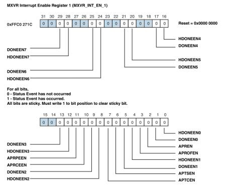
Figure 21-11. MXVR Interrupt Enable Register 1 (MXVR\_INT\_EN\_1)
