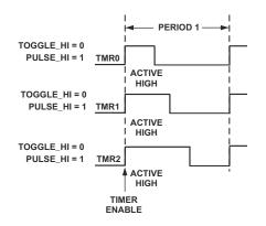
Figure 16-13. Timers With Pulses Aligned to Asserting Edge
