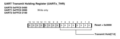
Figure 13-5. UART Transmit Holding Register
