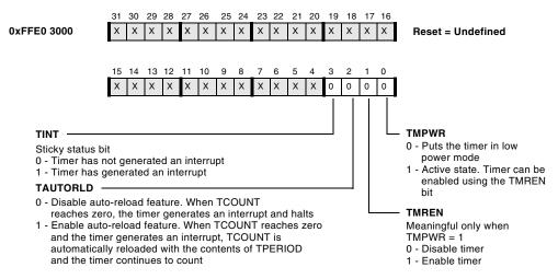
Figure 16-26. Core Timer Control Register
