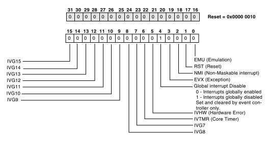
Figure 4-21. Core Interrupt Pending Register
