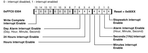
Figure 17-5. RTC Interrupt Control Register
