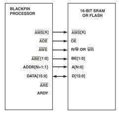
Figure 22-2. Interface to 16-bit SRAM or Flash
