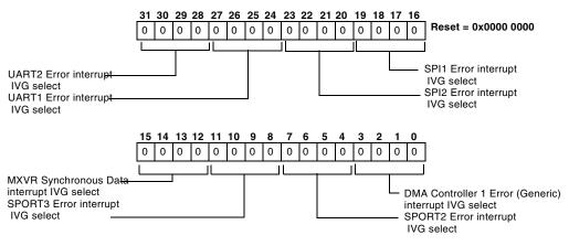
Figure 4-15. System Interrupt Assignment Register 3 (SIC\_IAR3)
