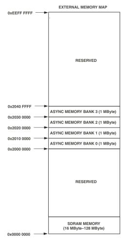
NOTE: RESERVED OFF-CHIP MEMORY AREAS ARE LABELED IN THE DIAGRAM ABOVE. ALL OTHER OFF-CHIP SYSTEM RESOURCES ARE ADDRESSABLE BY BOTH THE CORE AND THE SYSTEM.
