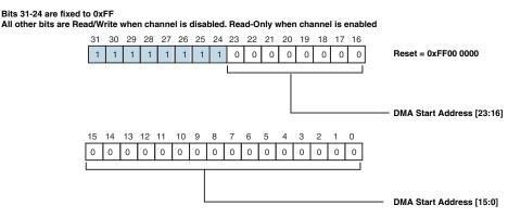
Figure 21-22. MXVR DMA Channel x Start Address Registers (MXVR\_DMAx\_START\_ADDR)
