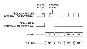
Figure 12-17. Example of TCKFE = RCKFE = 0, Transmit and Receive Connected
