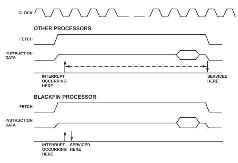
Figure 4-24. Minimizing Latency in Servicing an ISR
