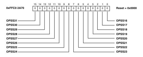
Overwrite Protection/Single Shot Transmission Register 2 (CAN\_OPSS2)
