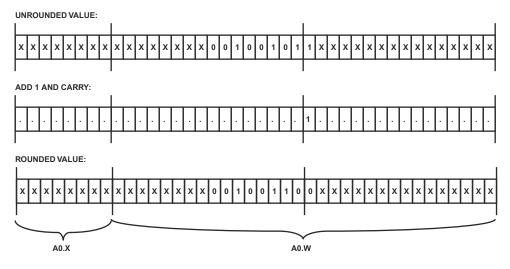
Figure 2-6. Typical Unbiased Multiplier Rounding
