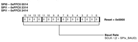
Figure 10-3. SPI Baud Rate Registers
