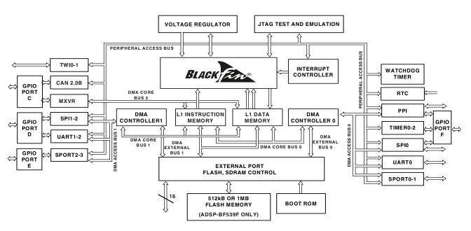
Figure 1-1. Processor Block Diagram
