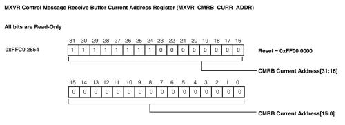
Figure 21-33. MXVR Control Message Receive Buffer Current Address Register (MXVR\_CMRB\_CURR\_ADDR)
