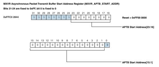
Figure 21-29. MXVR Asynchronous Packet Transmit Buffer Start Address Register (MXVR\_APTB\_START\_ADDR)
