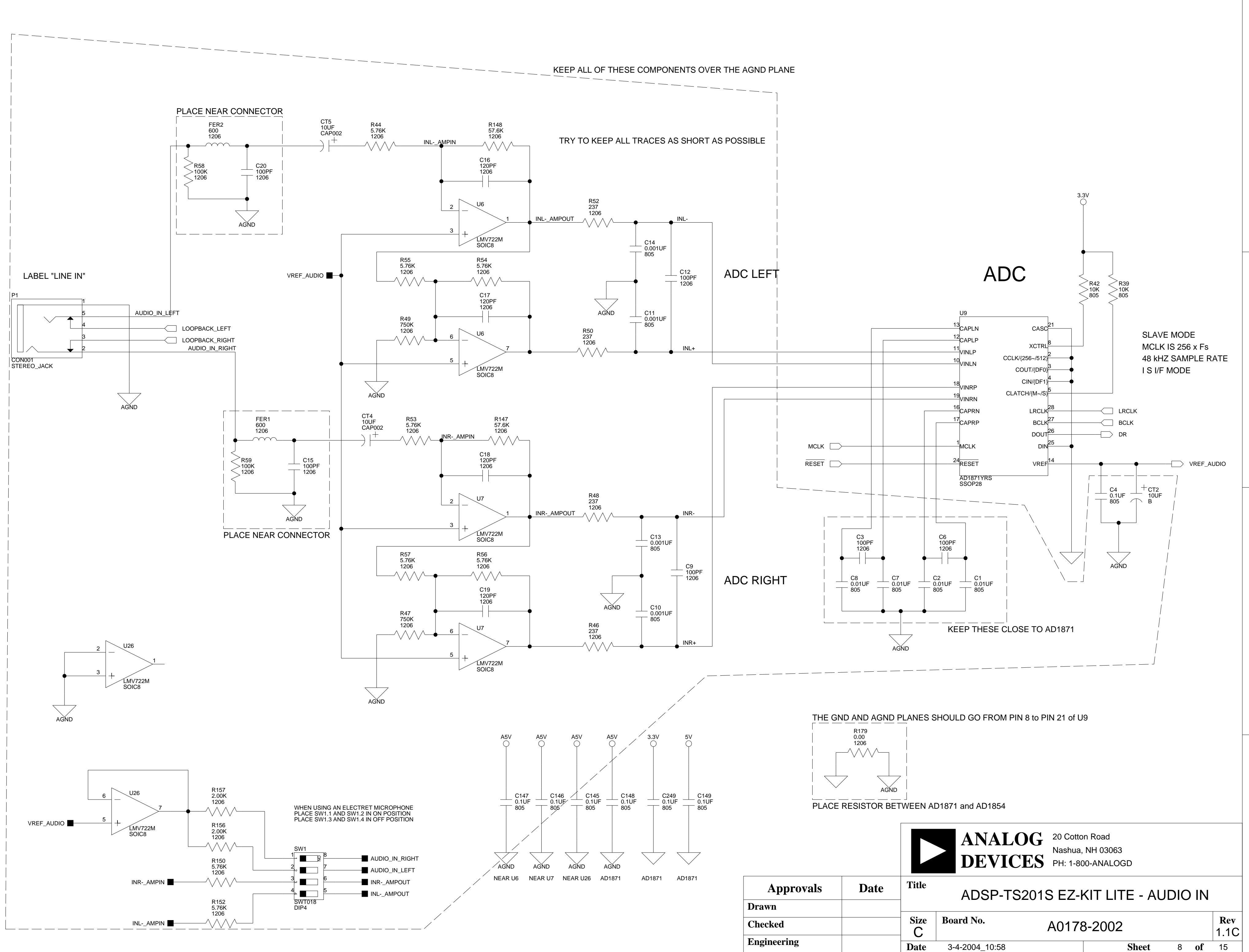
THE GND AND AGND PLANES SHOULD GO FROM PIN 10 to PIN 20 of U3
