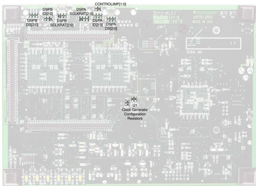
Figure 2-3. Resistor Locations (Bottom View of Board)
