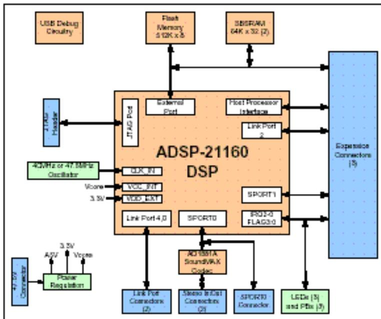
Figure 3-1. System Architecture Block Diagram
