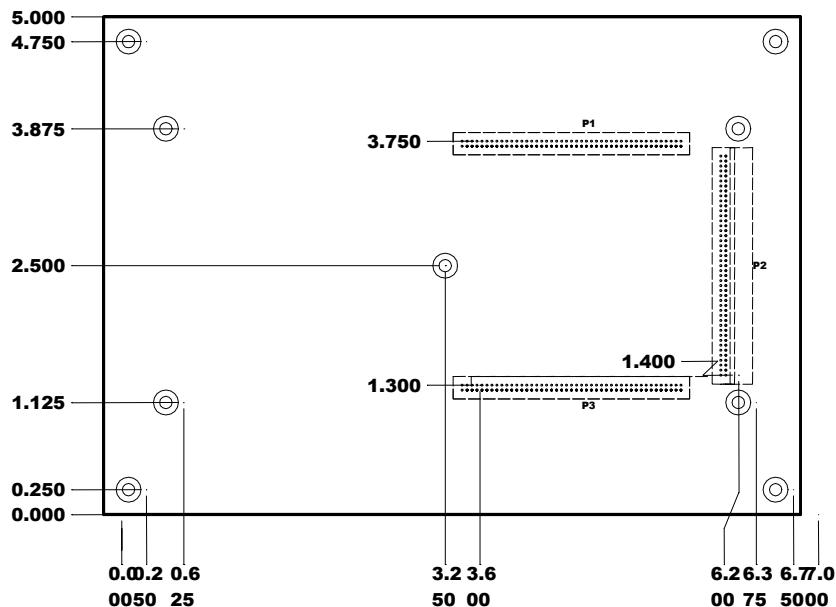
Figure 3-5. Mechanical Drawing
