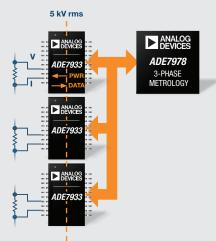
This integration enables the use of shunt resistor sensing elements instead of current transformers (CTs), thereby providing immunity to magnetic field interference and tampering. The use of shunts instead of CTs also reduces system cost and size.
