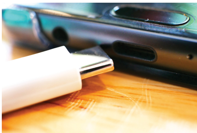
Figure 1. A cell phone with a USB Type-C connector for charging.
