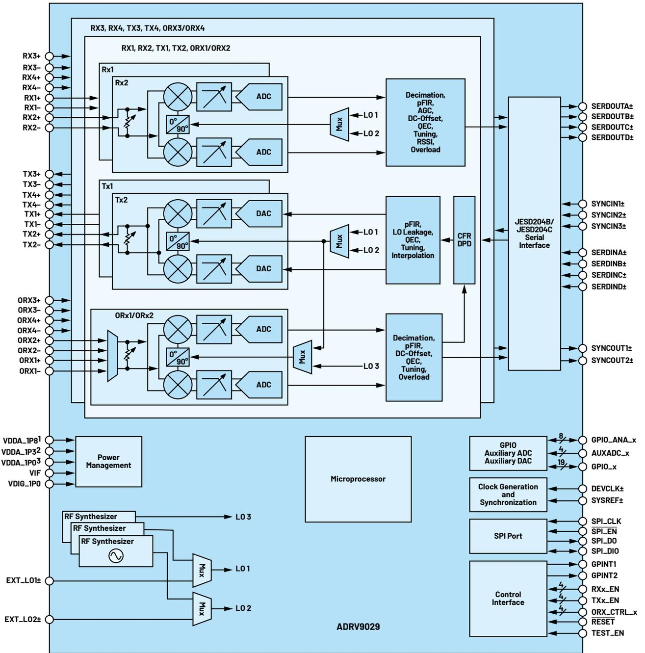
Figure 4. An ADR9029 functional block diagram.
