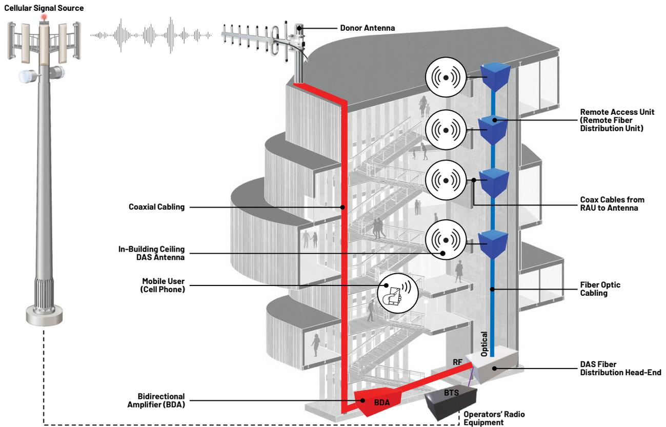
Figure 1. A hybrid DAS architecture.
