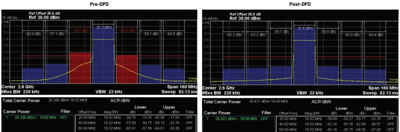
Figure 5. Power spectral density showing improvement in ACLR after application of DPD for a 20 MHz LTE signal.
