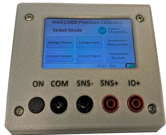
Figure 7. The MAX22000 precision calibrator in a 3D print case.
