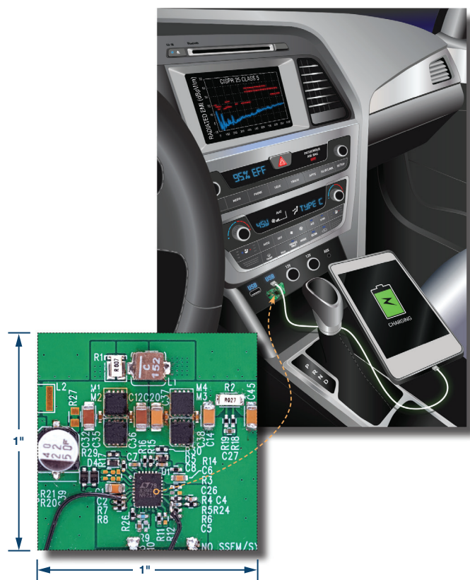
Figure 1. Efficient, low EMI USB Type-C power solution that fits in a 1" square.
