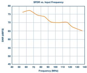
Figure 4. SFDR of the LTC2185 driven with the ADA4927-1.
