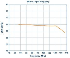
Figure 3. SNR of the LTC2185 driven with the ADA4927-1.
