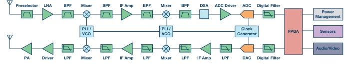
Figure 1. Basic superheterodyne architecture.
